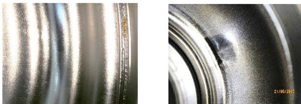
Figure 11: SPL #2 inner surface after 120  $\mu\text{m}$  EP. Left is the equator and right the iris with a noticeable mechanically polished area.
