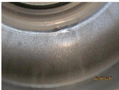
Figure 12: SPL #2 representative lower half cell after the 7<sup>th</sup> and 8<sup>th</sup> runs (170  $\mu\text{m}$  EP).
