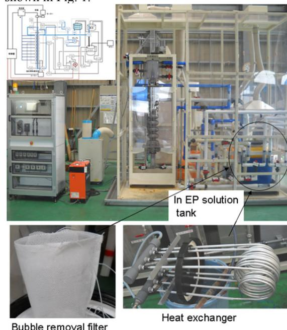
Figure 1: Pictures of facility and parts after improvement.
