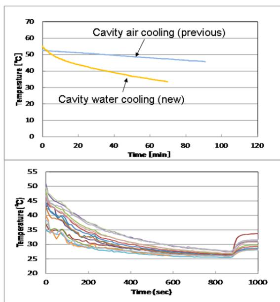
Figure 6: Results of hot water circulation test, (Upper) hot water temperature in cavity with air cooling and water cooling, (Lower) cavity surface temperature (15 points) during water cooling.
