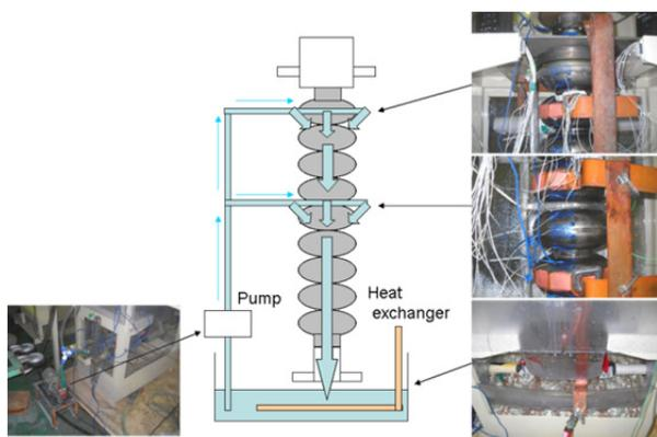
Figure 5: Pictures and schematic view of cavity water cooling system.
