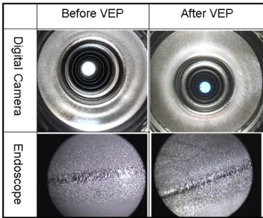
Figure 8: Images of inner surface observed with a digital camera and an endoscope.
