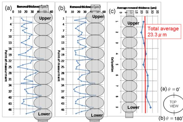
Figure 9: (a) Removal thickness of each part ( $\theta=0^\circ$ ) (b) Removal thickness of each part ( $\theta=180^\circ$ ) (c) Average removal thickness of each cell.
