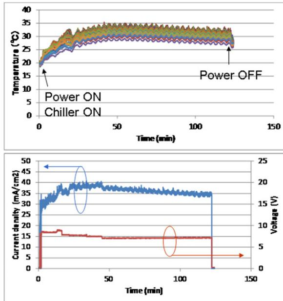
Figure 2: Logged data during VEP, (Upper) cavity temperature, (Lower) current density and voltage.
