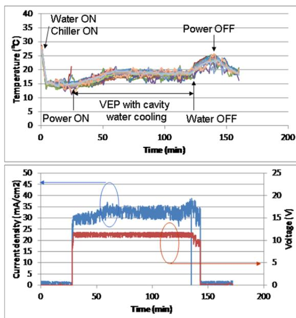
Figure 7: Logged data during VEP, (Upper) cavity temperature, (Lower) current density and voltage.
