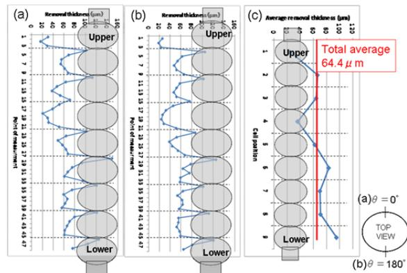
Figure 4: (a) Removal thickness of each part ( $\theta=0^\circ$ ) (b) Removal thickness of each part ( $\theta=180^\circ$ ) (c) Average removal thickness of each cell.
