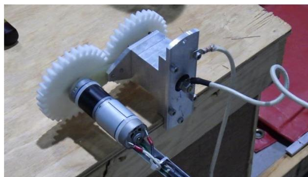
Figure 4: Rotary electrical contact and motor during load test.
