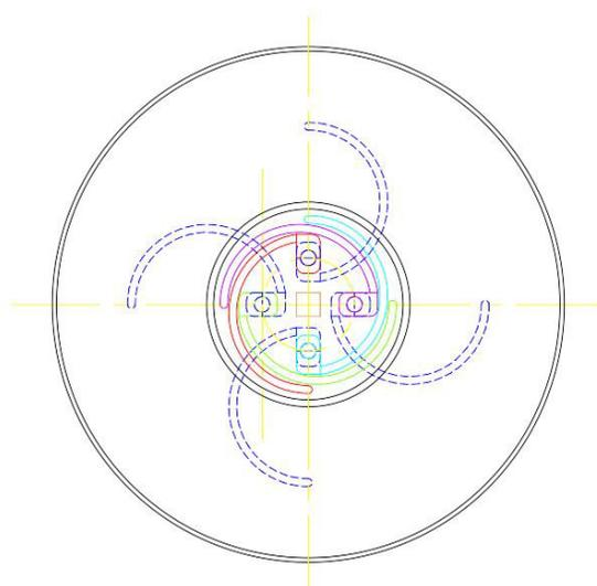
Figure 3: 2-dimensional drawing showing how the paddles would nest into one another to be able fit through the beam tube.
