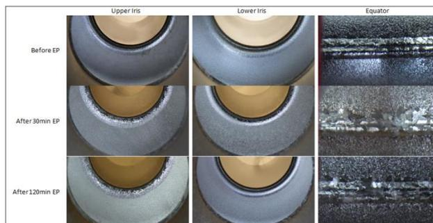
Figure 6: These pictures represent the different areas of the cavity after the first and second VEP experiments.
