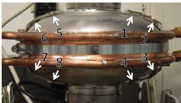
Figure 5: US probe fixture and positions.
