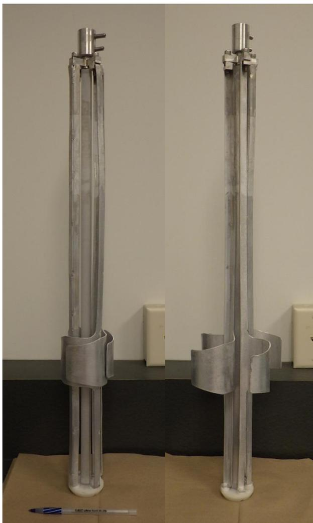
Figure 2: The cathode on the bench in both the closed and open configuration. Left-hand side: The cathode in the closed position. Right-hand side: The cathode in the open position.
