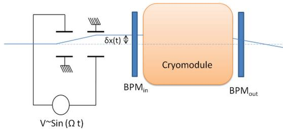
Figure 7: Potential setup for beam based HOM measurements. A pair of RF deflectors creates a modulation in the beam offset to the beam axis and excites a HOM if the modulation frequency matches to a HOM.
