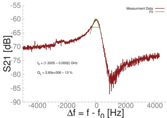
Figure 4: Fitting a Lorentz-curve to the resonance signal of the  $TM_{010}-\pi$  mode reveals the  $Q_L$ .
