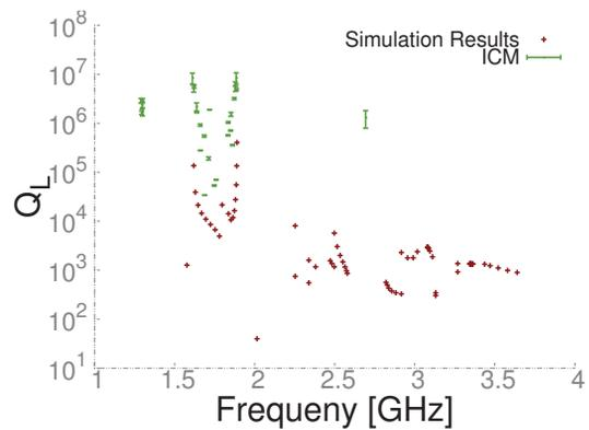
Figure 5:  $Q$  fitting results of the ICM compared to simulations show a difference for modes between 1.5 and 2 GHz of 2 orders of magnitude in  $Q_L$ .
