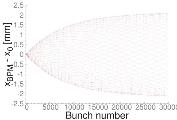
Figure 8: Simulated bunch position after the beam gets kicked by HOM in the ACM cryomodule.
