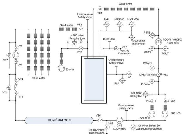
Figure 3: Sketch of the cryostat vacuum connections.
