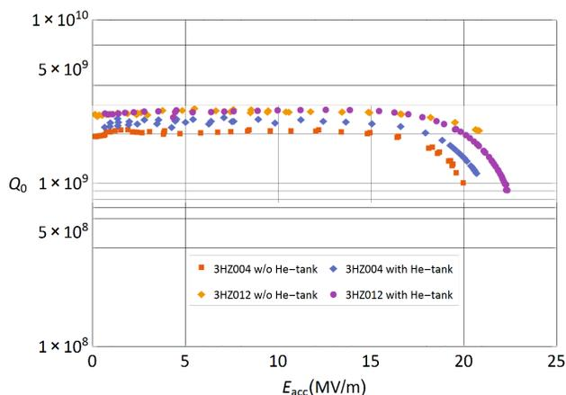
Figure 10: Power rise comparison for cavity 3HZ004 and 3HZ012 before and after He-Tank integration.
