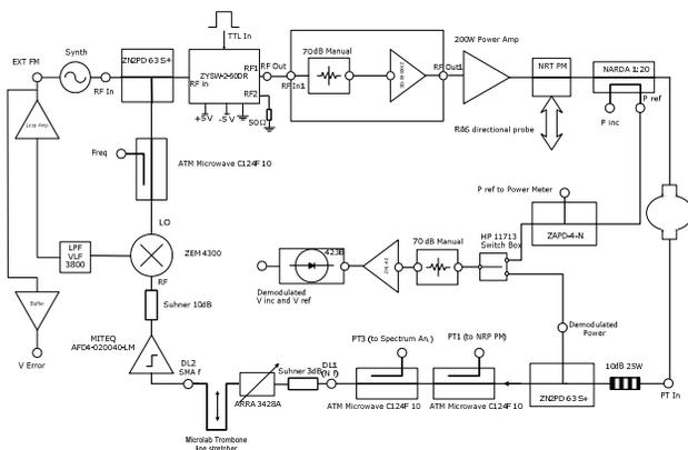
Figure 5: Block diagram of the 3.9 GHz cavity PLL.
