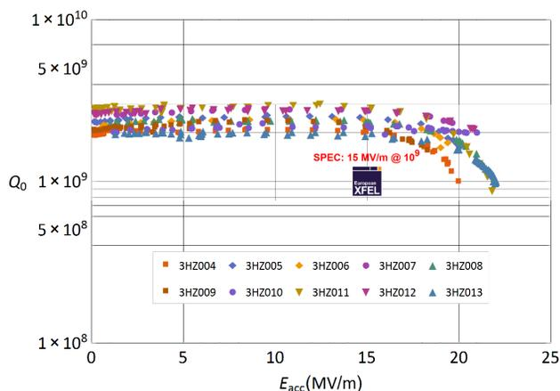
Figure 7: Summary plots for power rises of the ten E-XFEL 3.9 GHz cavities at 2 K.
