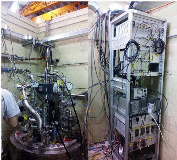
Figure 2: Inside views of the Vertical Test bunker: on the left, top flange of the cryostat with connections for RF, thermometers and vacuum; on the right, cabinet hosting electronics for signal processing and RF.
