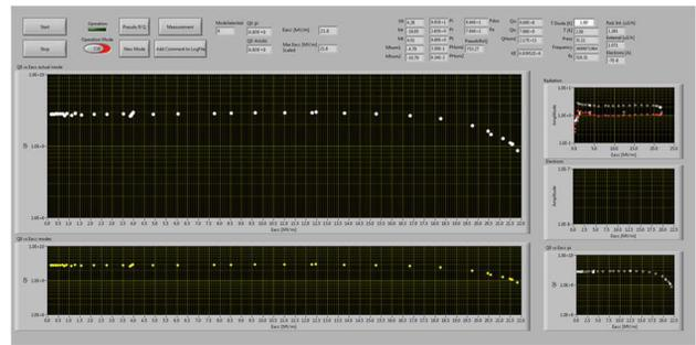
Figure 6: Typical power rise acquired from the LabVIEW™ Control Panel. In the same panel, other parameters are displayed such as radiation level on top of the cryostat (upper plot on the left).
