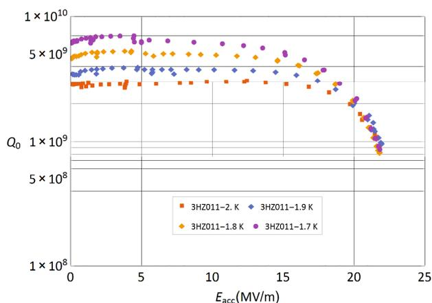
Figure 8: 3.9 GHz power rises at different temperatures for cavity 3HZ011.
