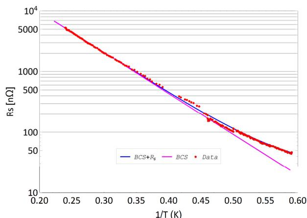
Figure 9: 3.9 GHz cavity resistance versus He bath temperature.
