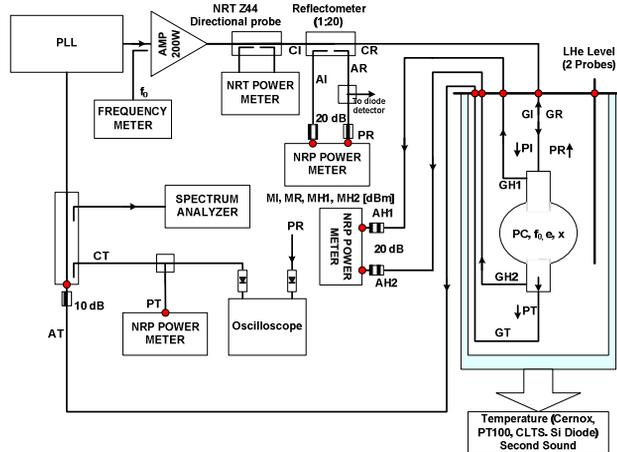
Figure 4: Block diagram of the RF system used for test 3.9 GHz cavity.
