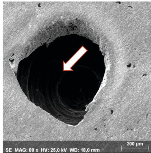
Figure 7: SEM image of the coupon surface around the off-axis hole indicating shearing and lamination of the upper surface layer.
