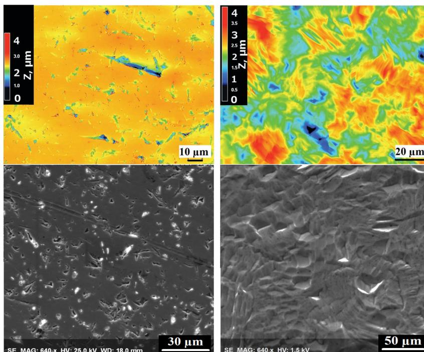
Figure 9: Laser scanning (top) and SEM (bottom) images of the CBP sample before (left) and after (right) 20  $\mu\text{m}$  additional BCP polishing.
