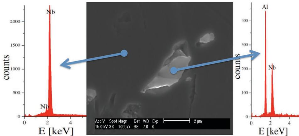
Figure 5: Al<sub>2</sub>O<sub>3</sub> inclusions found embedded in the Nb surface as identified by SEM/EDX analyses on the CBP sample from the tube area.
