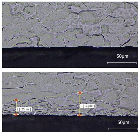
Figure 8: Laser scanning microscopy images of the cross-sections of the initial coupon-material (top) and after four-step CBP polishing (bottom) revealing a surface damaged layer (bottom side of the cross-sections).
