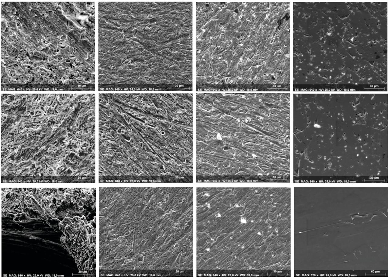
Figure 4: SEM images of the surface of niobium coupons after step 1 to 4 (from left to right column correspondingly) polished in the location of the end tube (upper), tapered cell area (middle), and equator area (lower row).
