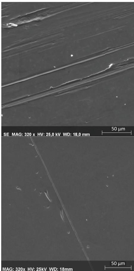
Figure 6: SEM images of the equator surface before (top) and after (bottom) renewal of the polishing media at the final polishing step.
