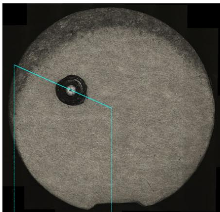
Figure 3: Front-side view of the coupon-sample (diameter 8.6 mm) with an off-axis pit for the determination of the removal rate.
