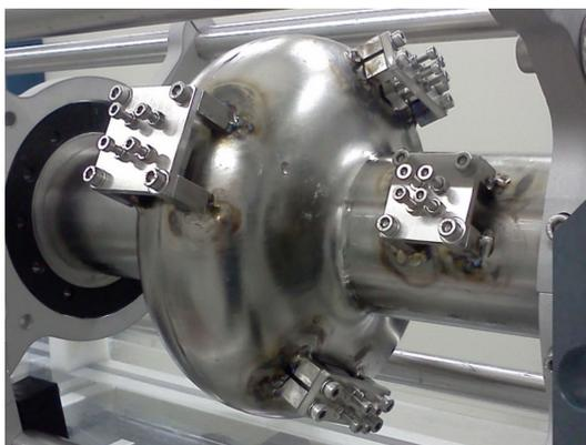
Figure 2: Coupon cavity used for the characterization of the CBP polishing. The protruding structures indicate the position of the removable samples.
