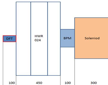
Figure 5: A periodic section for CM2 and CM3.
