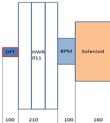
Figure 3: A periodic section for CM0 and CM1.
