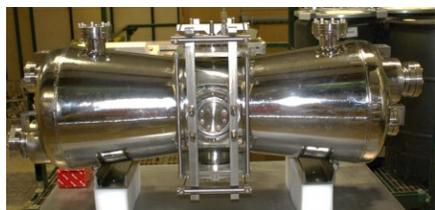
Figure 4: 162.5 MHz half wave resonator.
