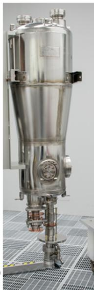
Figure 3: 72.75 MHz quarter wave resonator.
