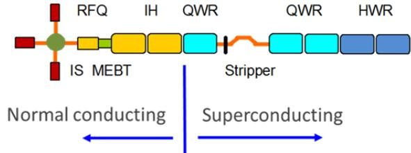
Figure 1: A schematic drawing of the MEIC ion linac.
