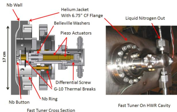
Figure 7: Fast piezo-electric tuner example for QWRs and HWRs.
