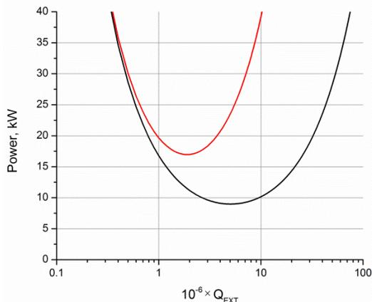
Figure 6: Required RF power for the QWR as a function of the external Q-factor when the microphonic detuning is controlled by piezotuners (black) and by additional RF power (red).
