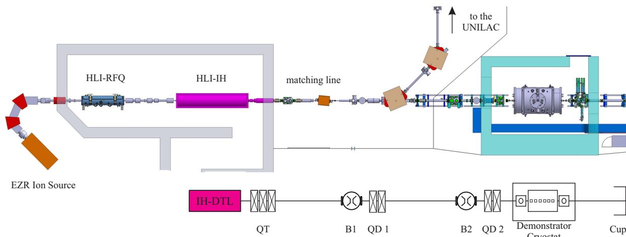
Figure 1: Top: footprint of the demonstrator test environment at GSI. Bottom: scheme of the beam line. The main elements of the beam line: quadrupole triplet QT, quadrupole doublets QD1 and QD2 and two buncher cavities B1, B2.
