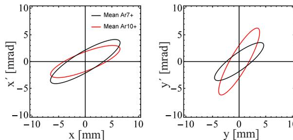
Figure 4: Comparison of averaged phase space ellipses for  $Ar^{10+}$  and  $Ar^{7+}$  beams.
