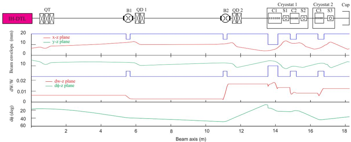
Figure 5: Top: preliminary layout of the first stage of the advanced demonstrator. Bottom: calculated transverse and longitudinal beam envelopes.
