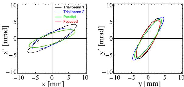
Figure 3: Backwards calculated phase space ellipses to the output of IH-DTL for four different sets of gradients for  $Ar^{10+}$  beam.
