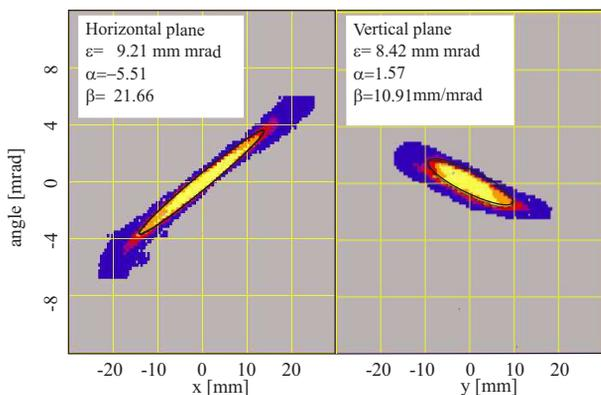
Figure 2: Example of measured emittance for  $Ar^{10+}$ . The black curves show  $4 \cdot \epsilon_{rms}$  phase space ellipses.
