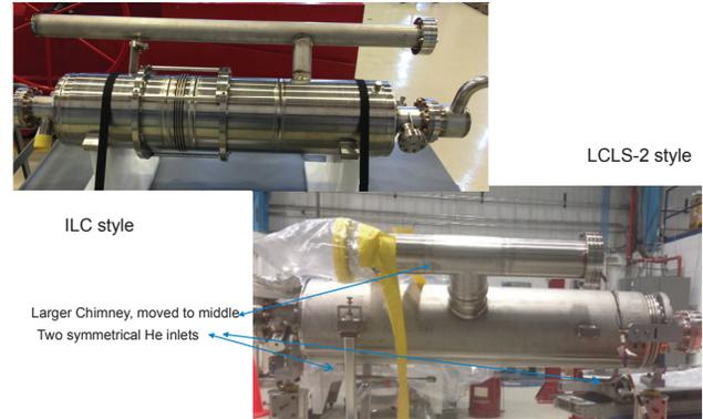
Figure 6: Comparison of the two different styles of Ti vessels used – ILC and LCLS-2.
