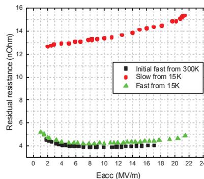
Figure 4: Residual resistance obtained from the deconvolution of surface resistance for the three different cooldowns, revealing the trapped flux induced residual resistance changes.
