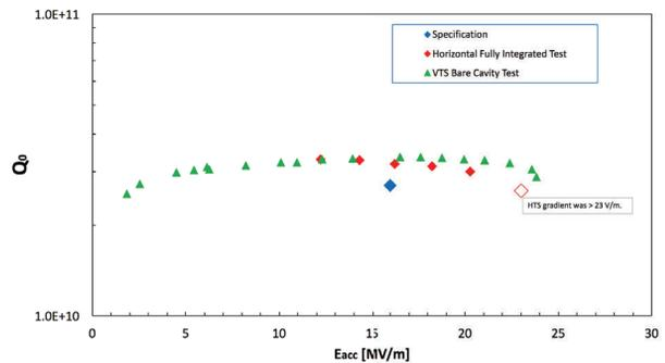
Figure 7: Record Q > 3e10 at 16MV/m, 2K for a LCLS-2 dressed cavity in fully integrated horizontal test (with high power coupler, HOMs, tuner etc).
