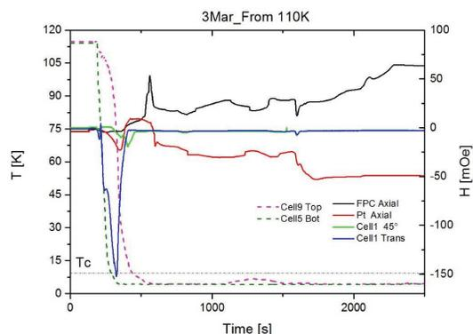
Figure 12: Large thermoelectrically induced field ~ 150 mGauss returning to ~zero after cavity transition, indicating that close to none of the transient field was trapped at the cavity surface.
