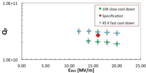
Figure 8: Fast versus slow cooldown results of record LCLS-2 N doped dressed nine cell TB9AES021 in dressed horizontal test with < 4 mGauss field.
