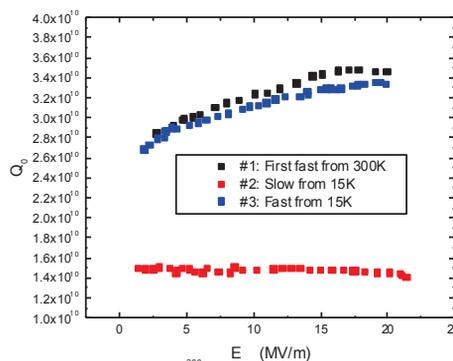
Figure 3: Slow vs fast cooling vertical test results for the dressed N doped nine cell TB9AES011.
