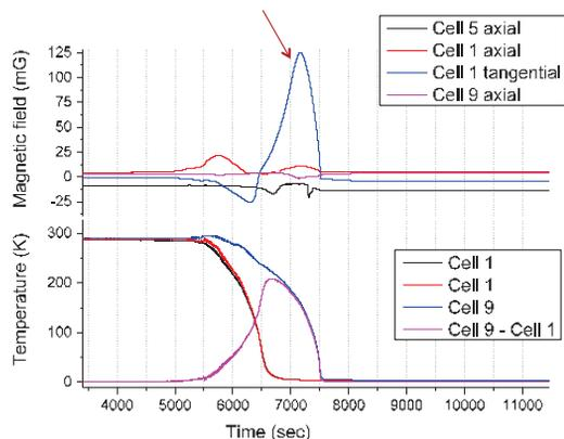
Figure 2: Magnetic field at the cavity surface (longitudinal and transverse) recorded during cooldown in the vertical test dewar from 300K.
