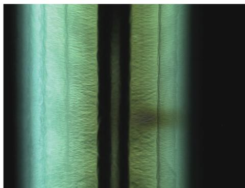
Figure 5: Heavy oxidation encountered at irises of some of the dressed cavities. Darker localized spots are noticed.
