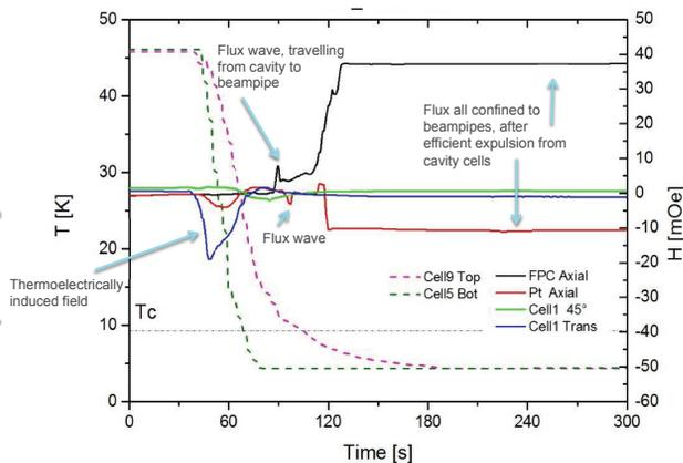
Figure 9: Temperature and magnetic field recordings during a cavity cooldown from 45K.
