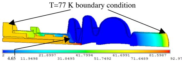
Figure 6: Temperature distribution, K.
