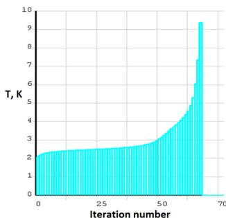
Figure 2: 1D model temperature rise during quench.
