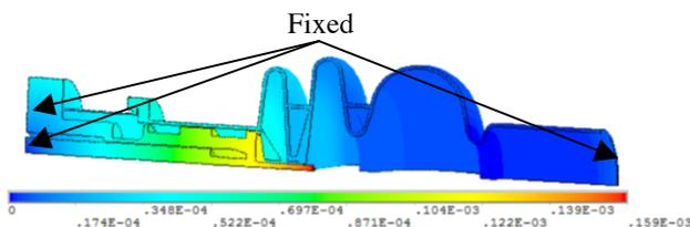
Figure 8: Temperature deformations, m.
