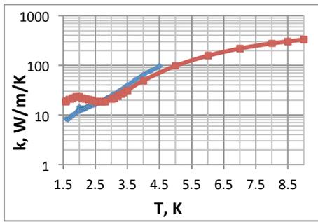
Figure 1: Thermal conductivity coefficients of Nb RRR300 for different crystal structures from Wah Chang measured at Fermilab [3]: red curve - large grain, blue curve – fine grain.
