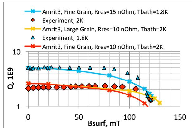
Figure 4: 3.9 GHz 9 cell QvsB curves.
