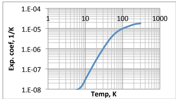
Figure 9: Copper thermal expansion coefficient.
