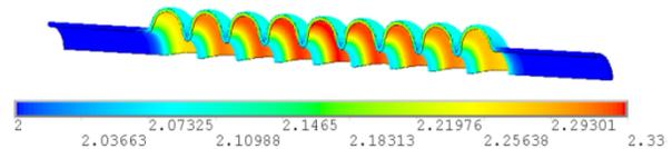
Figure 3: 3.9 GHz 9 cell cavity temperature distribution just before the quench (Fine grain, Amrit3, Rres=10nOhm).
