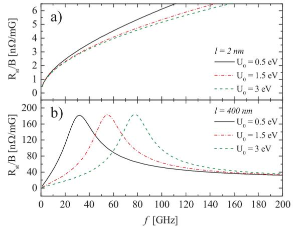
Figure 4: Resistance per mG of trapped field for different pinning potentials as a function of the frequency, for the dirty a) and clean b) limits respectively.
