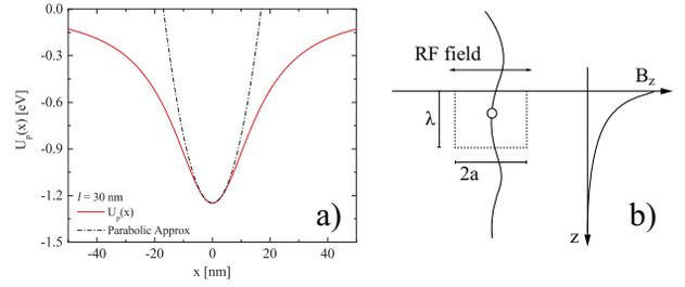
Figure 1: a) Lorentzian pinning potential and its parabolic approximation, b) sketch of the oscillating vortex pinned at the RF surface.
