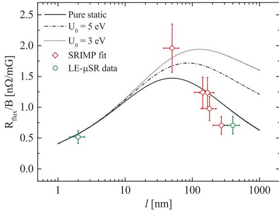
Figure 3: Experimental resistance per unit of trapped field data acquired for 1.3 GHz SRF cavities [4]. The three lines correspond to the simulations: solid line for pure static dissipation, dashed-dotted and dotted lines for total flux resistance calculated with two different pinning potentials.
