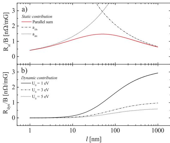
Figure 2: Resistance per mG of trapped magnetic field as a function of the mean free path: a) only static resistance, b) only dynamic resistance for different pinning potentials  $U_0$ .
