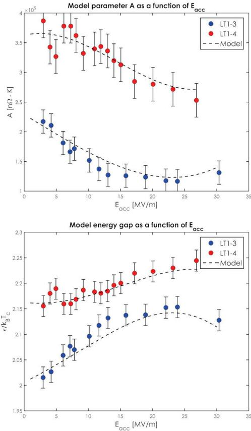
Figure 2: **Top:** The pre-exponential factor  $A$  vs.  $E_{acc}$ . The model curves are also included. The effective energy gap is fixed. **Bottom:** Effective quasi-particle energy gap,  $\epsilon/k_B T_c$  plotted against  $E_{acc}$  along with the corresponding model ( $T_c = 9.28$  K for LT1-3 and 9.22 K for LT1-4). The pre-exponential factor  $A$  is fixed.
