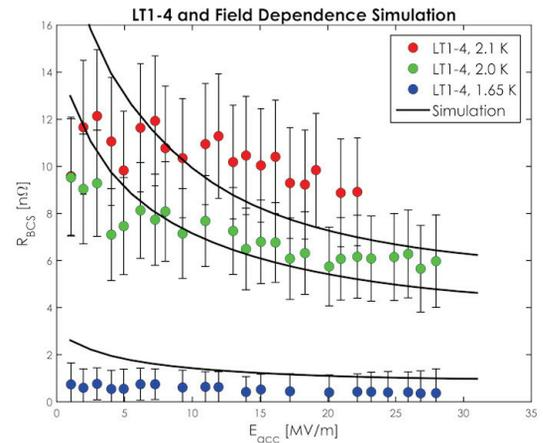
Figure 5:  $R_{BCS}$  vs.  $E_{acc}$  with field dependent BCS simulation based on [6] using material parameters obtained at low fields. Simulation agrees well with the experimental data for LT1-3 but disagrees with data from LT1-4.
