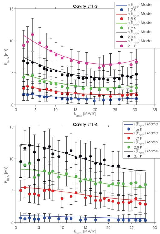
Figure 3:  $R_{BCS}$  vs.  $E_{acc}$  with model curves letting the effective energy gap vary while assuming a fixed mean free path using SRIMP to model BCS theory.
