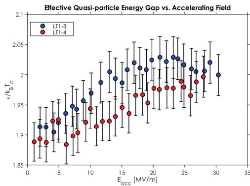
Figure 4: Effective quasi-particle energy gap vs.  $E_{acc}$  using SRIMP to extract the effective gap values.
