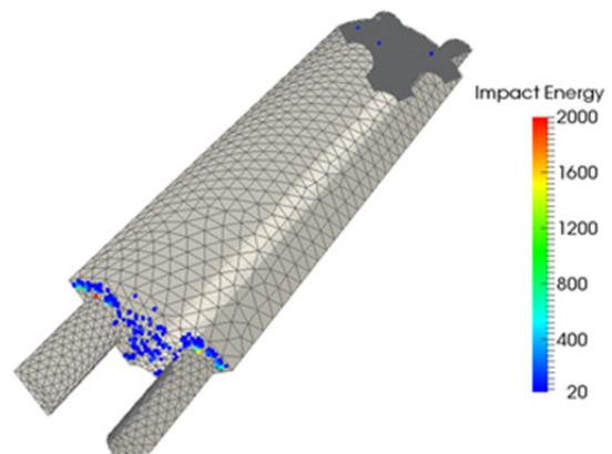
Figure 4: Resonant particles on cavity surface.
