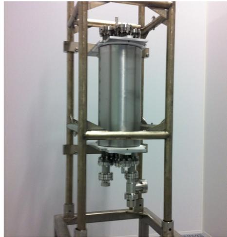
Figure 8: Prepared cavity for a cryogenic test in the clean room.
