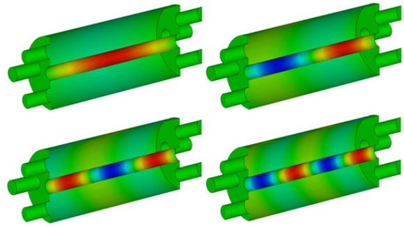
Figure 2: Cavity showing surface electric field distribution from top left clockwise TEM1, TEM2, TEM3, and TEM4.
