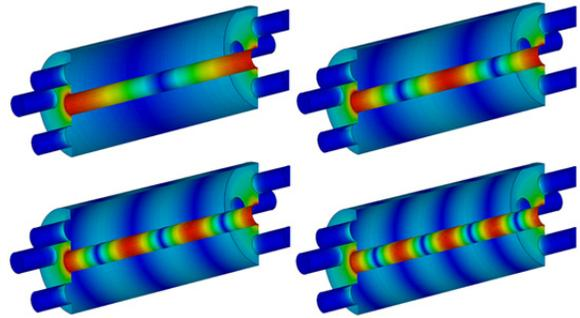
Figure 3: Cavity showing surface magnetic field distribution from top left clockwise TEM1, TEM2, TEM3, and TEM4.
