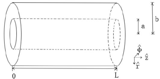
Figure 1: Coaxial half wave resonator.
