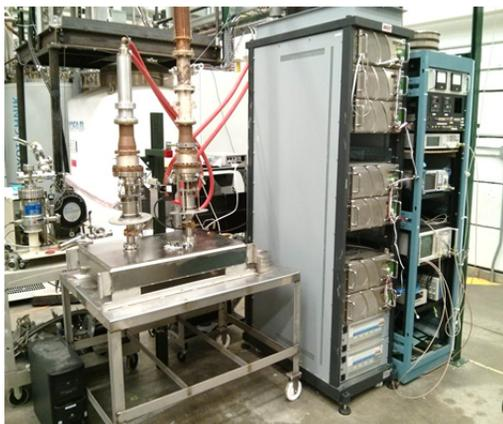
Figure 13: RF conditioning system for HWR couplers.
