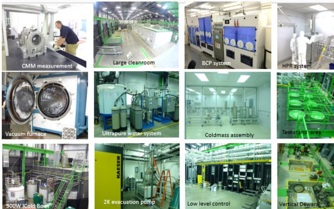
Figure 24: Infrastructures in SRF Highbay: from top left to right CMM measurement (dimensional inspection), large clean room for cavity assembly, BCP system for cavity processing, PR system. From middle left to right, Hydrogen degassing vacuum furnace, Ultrapure water system, coldmass assembly area, test stand area. From bottom left to right, 900W cold box, 2 K helium gas evacuation pump, Low level control area, vertical Dewars for cavity certification test.
