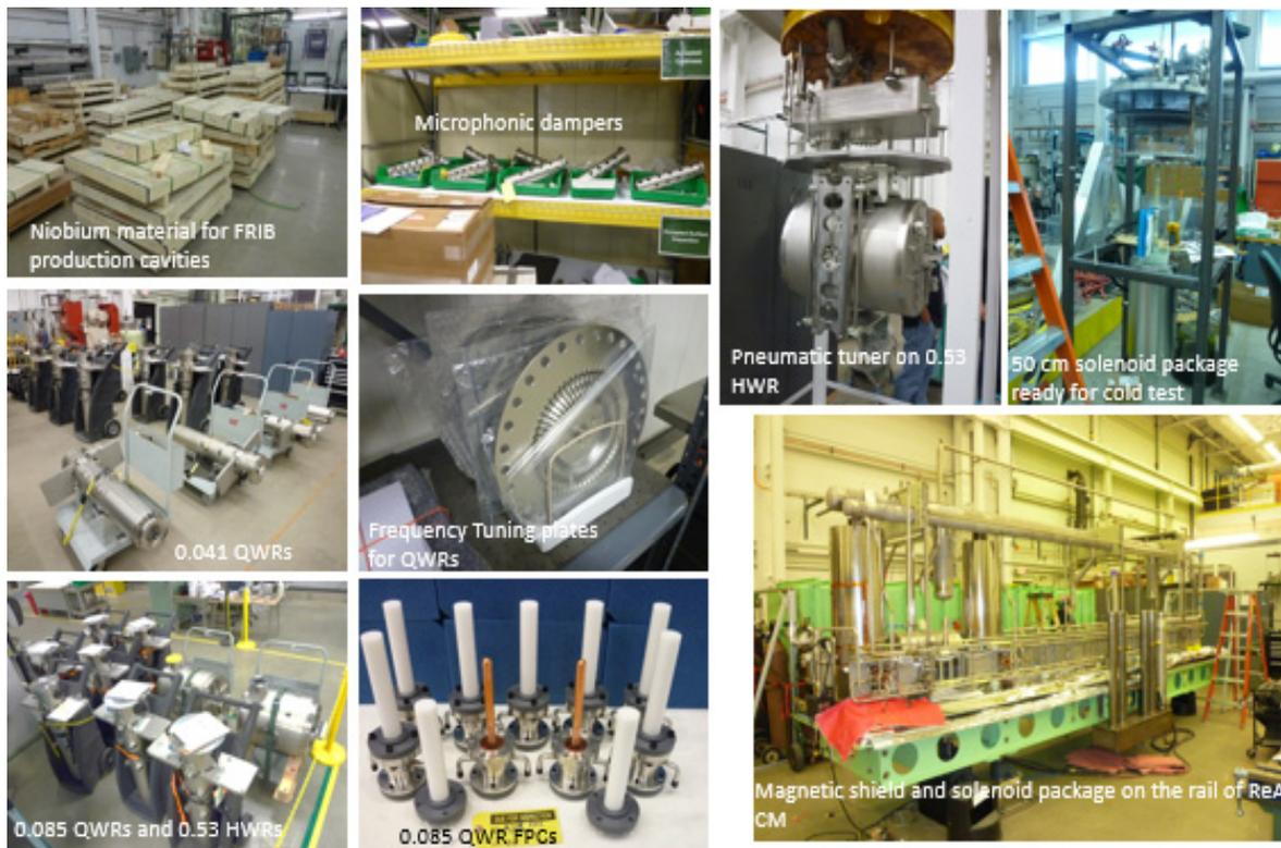
Figure 23: Some examples of recent deliveries. From top left to right, niobium materials, dampers for QWRs, HWR pneumatic tuner, 50 cm superconducting solenoid package. From middle left to right 0.041QWRs, tuning plate for QWRs. From bottom left to right, 0.041/0.085QWRs and 0.53HWRs, FPCs for 0.085QWRs, magnetic shield on the 0.085QWRs (ReA6-1).
