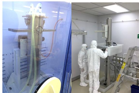
Figure 7: Left, BCP for 0.041 QWR at SRF Highbay facility, Right, HPR in the SRF clean room.
