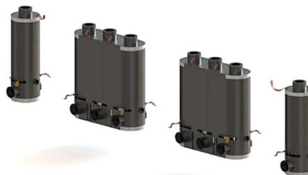
Figure 18: Magnetic shield design of ReA3/ReA6.
