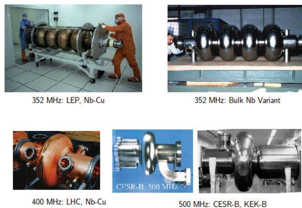
Figure 8: A select set of SCRF cavities already used in high current storage ring including LEP (top), LHC, CESRB and KEKB (bottom).
