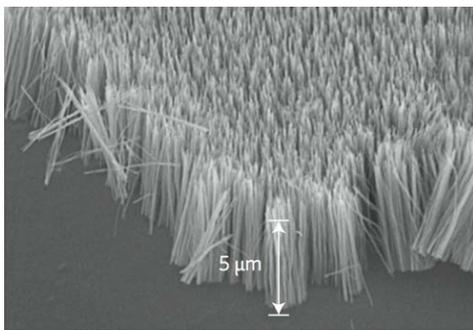
Figure 11: CSU developed conductive 15  $\mu\text{m}$  long Nickel nanowires. The interior of the array is very uniform. Our intent is to attempt to use this technology to create nanowires of Nb.
