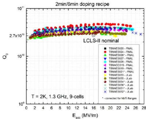
Figure 5:  $Q_0$  vs  $E_{acc}$  for N-doped 1.3 GHz 9-cell cavities. The average  $Q_0$  is  $> 3 \times 10^{10}$ . Process confirmed at FNAL, Jefferson Lab, and at Cornell.
