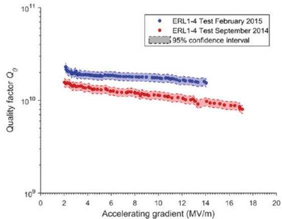
Figure 8:  $Q_0$  vs  $E$  plot for an Nb 1.3 GHz single cell cavity coated with Nb<sub>3</sub>Sn at Cornell. The cool-down procedure was improved between the tests, which results in a higher quality factor and reduced  $Q$ -slope.
