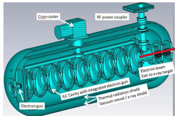
Figure 1: Overview of the proposed compact SRF accelerator. The overall length is 1.5 M with a diameter of < 0.5 M. For simplicity, no cavity magnetic shield is shown. Tuners are not needed since the RF system will be designed to lock to the cavity resonant frequency.
