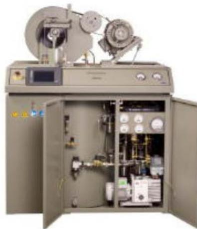
Figure 3: Commercial 4K refrigerators like this small machine made by Linde are excellent for many applications, but have cold boxes that use pistons or turbo expanders that are sensitive to contamination, require regular maintenance, and are physically large. They also depend on significant external infrastructure as illustrated in Figure 2.
