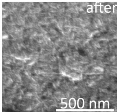
Figure 13: SEM images, typical for nitrogen-incorporated ultra-nano-crystalline diamond, (N)UNCD films, on Mo/SS after high power testing [16].
