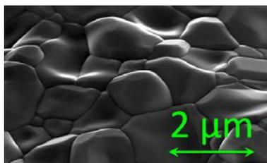
Figure 9: SEM image of Nb<sub>3</sub>Sn surface SEM indicates appropriate grain size and texture. EDX shows desired tin content for highest T<sub>c</sub> and confirms uniformity.
