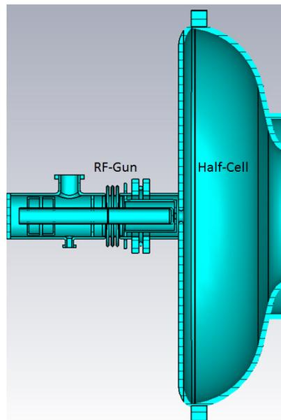
Figure 10: Schematic drawing of the electron gun with thermionic cathode that can be integrated into a multi-cell 1.3 GHz elliptical cavity. The thermionic cathode consumes 3 W leading to an estimated heat load from the cathode to the cavity cold surface at 4.5K of 0.1 W.
