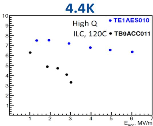
Figure 6:  $Q_0$  vs  $E_{acc}$  for non-optimized N-doped 1.3 GHz cavities at 4.4 K. The  $Q_0$  falls slowly with gradient and is  $\sim 6-7 \times 10^8$  at 6 MV/m (maximum gradient was limited by the coupler vs by quench.)
