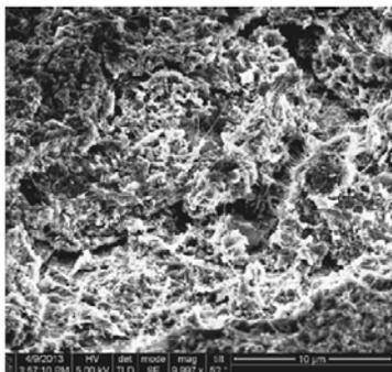
Figure 12: SEM micrograph of carbon nanotubes (CNT) used in a FE cathode built and tested by Radiabeam Technology, Fermilab and NIU [15].
