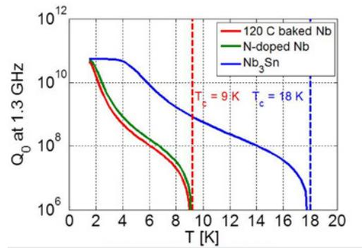
Figure 7: Calculated  $Q_0$  comparison between a pure Nb cavity and an Nb cavity coated with Nb<sub>3</sub>Sn at Cornell. Note  $Q_0$  increase by a factor of  $\sim 30$  at  $\sim 4.2$  K. (S. Posen, private comm.)
