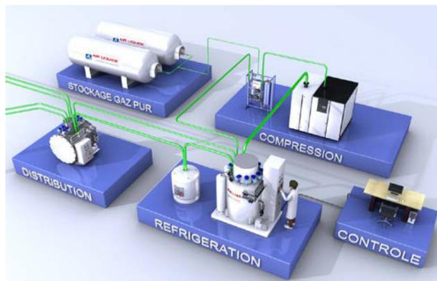
Figure 2: Typical commercial 4K refrigerators or liquifiers are elegant but complex requiring many external systems such as compressors, water cooling, electrical infrastructure, LN2 and LHe storage vessels, He gas storage and recovery systems, a He purification system, extensive piping, etc [9]. System maintenance and reliability are always an issue.
