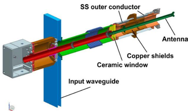
Figure 14: Cut view of low heat leak fundamental power coupler.
