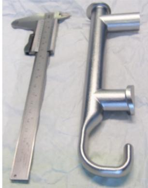
Figure 15: First prototype of the DQW HOM hook built at CERN.
