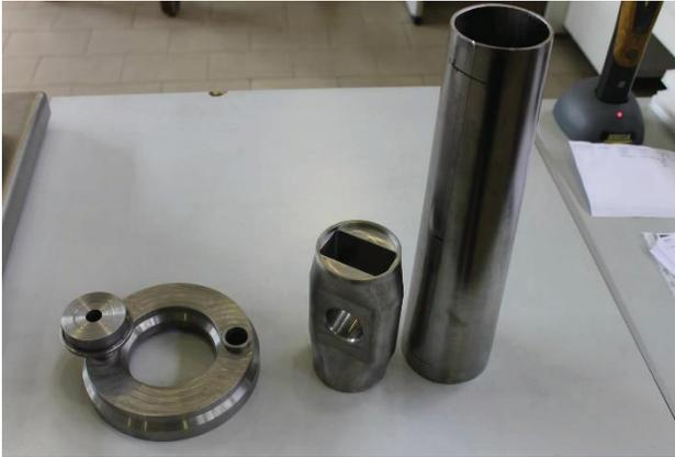
Figure 18: From left to right, cavity torus with one HPR port, central drift tube, conical stem.
