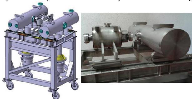
Figure 14: On the left, cavity string assembly test bench. On the right, Dummy HWR cavity solenoid and support frame (slightly longer than one eighth of the actual one).
