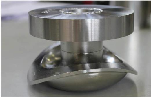
Figure 17: Preassembly of a beam port.
