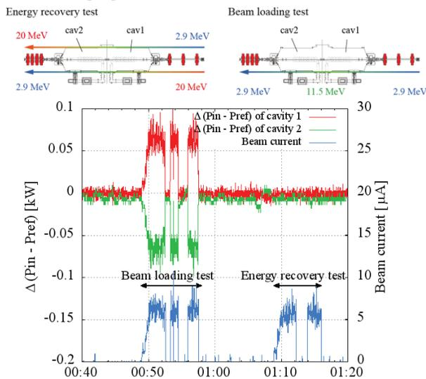
Figure 6: Energy recovery trial. Beam loading effect cannot be seen on “Energy recovery test”. In the “Beam loading test”, upper and lower cavity only accelerates and decelerates electron beams.
