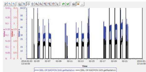
Figure 9: History of radiation status, monitored by ALOKA monitors, during cERL beam operation for three weeks at February of 2014. Radiation increased at February 14 in 2014. Spikes at the beginning of dairy operation are due to RF aging.
