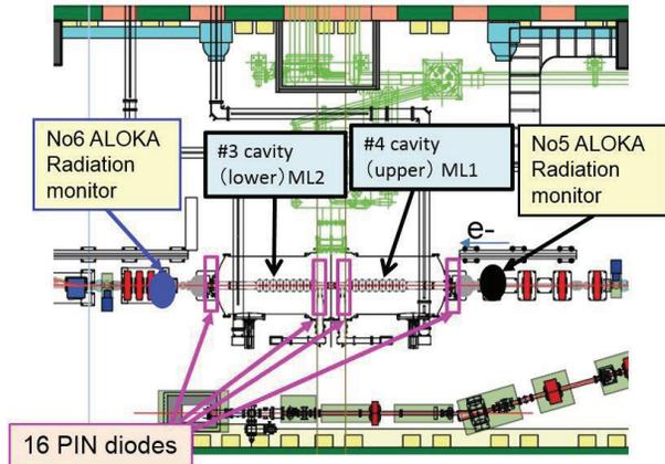
Figure 7: Setup of radiation monitors at cERL main linac cryomodule.
