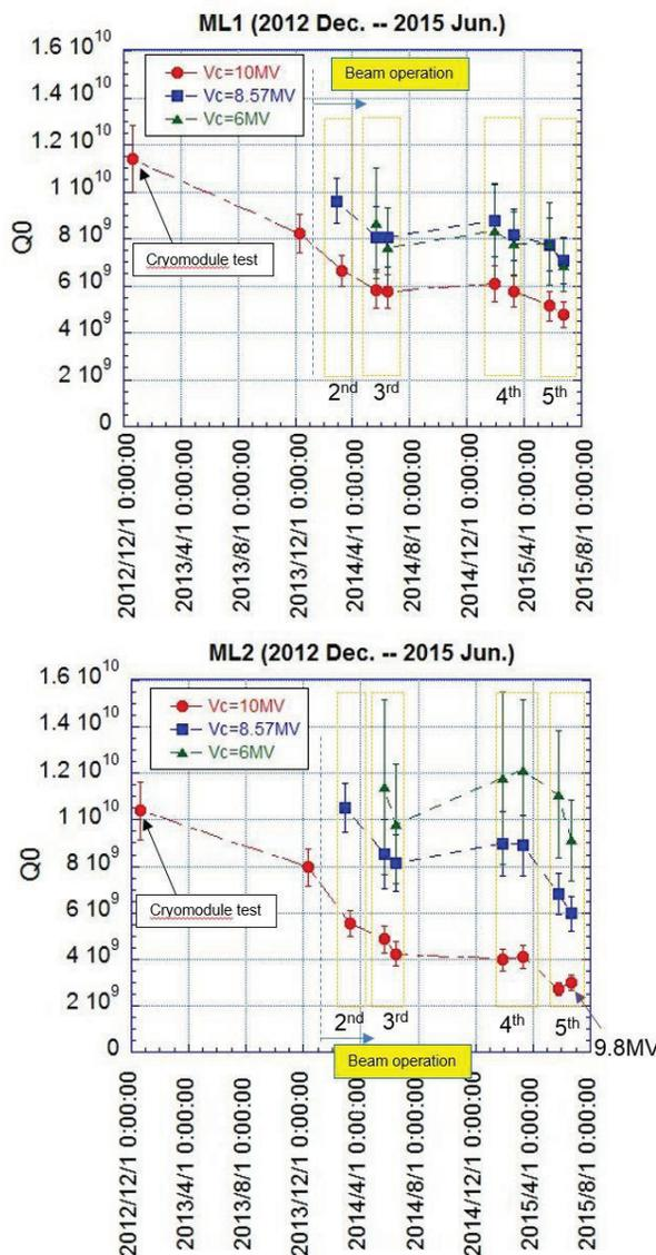
Figure 13: Measurement of the cavity performances of 6, 8.57 and 10 MV cavity voltage during long-term beam operation including cryomodule test of ML1 upper cavity (top) and ML2 lower cavity (bottom). Red, blue and green points are for 10MV, 8.57MV and 6MV, respectively except for the final red circle of 9.8 MV. Dotted boxes show the beam operation phases.
