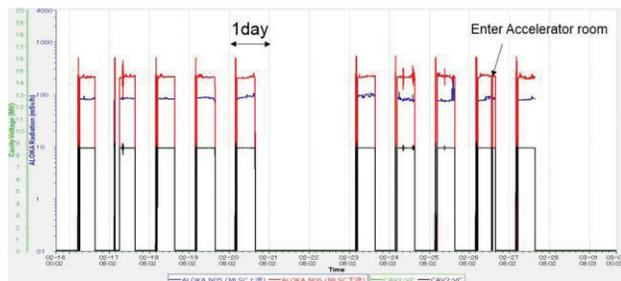
Figure 12: 2 weeks cavity voltages with radiation. Green (black) line shows the upper (lower) cavity voltage. Blue (red) line shows the measured radiation by upper (lower) ALOKA monitor. Spikes at the beginning of dairy operation are due to RF aging. Once we enter the accelerator room to check beam monitor.
