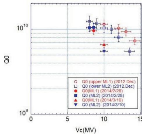
Figure 10: Q-values vs acceleration voltage. Red and blue points are for upper and lower cavities, respectively. Open circles (squares) show the measured data of high power test in 2012. Solid circles (squares) show the measured data during beam operation at 2<sup>nd</sup> phase in 2014. The Q-values were degraded during beam operation period.
