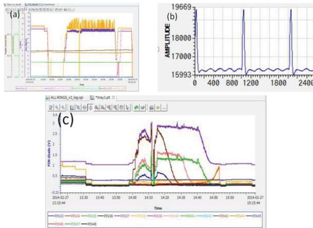
Figure 11: (a) RF field during pulse processing and (b) its magnification. (c) Decrease of radiation signal, observed by Si PIN diodes, during pulse processing.
