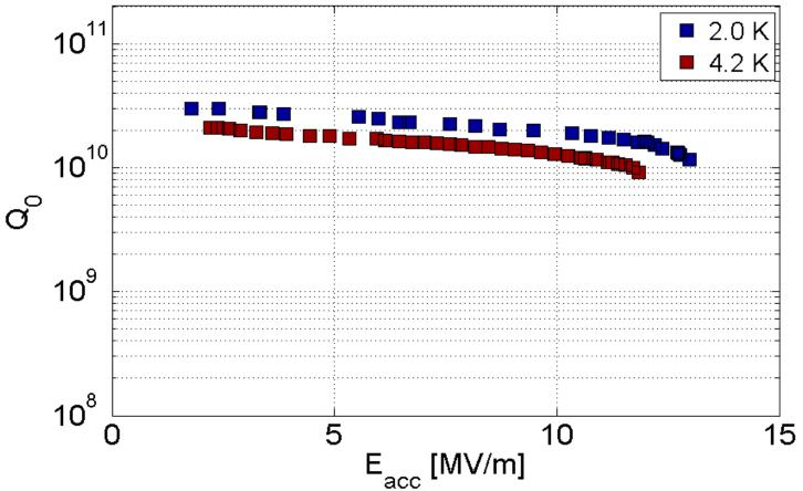
First accelerator cavity made with an alternative superconductor that outperforms Nb at usable gradients!
