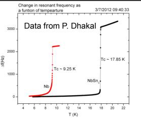
Transition temperature is  $\sim$  17.85 K. The best of three samples shows very smooth surface with no residual tin contamination
