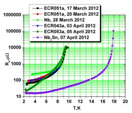
Recent measurements of surface resistance of several ECR films, bulk Nb sample, and Nb<sub>3</sub>Sn sample as a function of temperature at 7.4 GHz.
