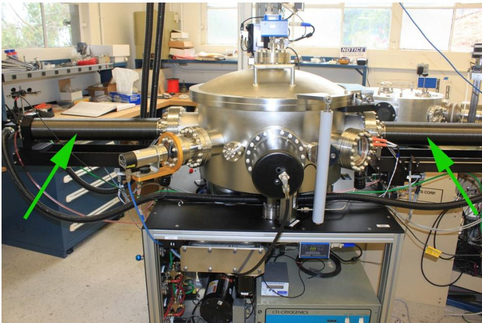
Dual Magnetron: Most effective for a Biasing & influencing Ion Energies and Trajectories
