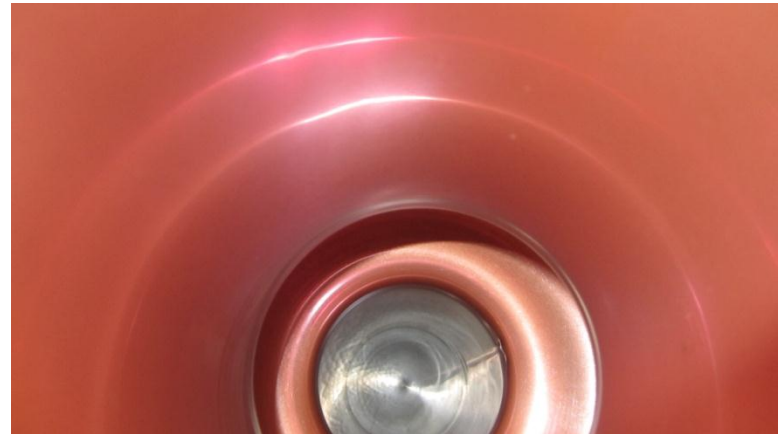
40 hours -40nm colloidal silica and wood blocks - oxidized
