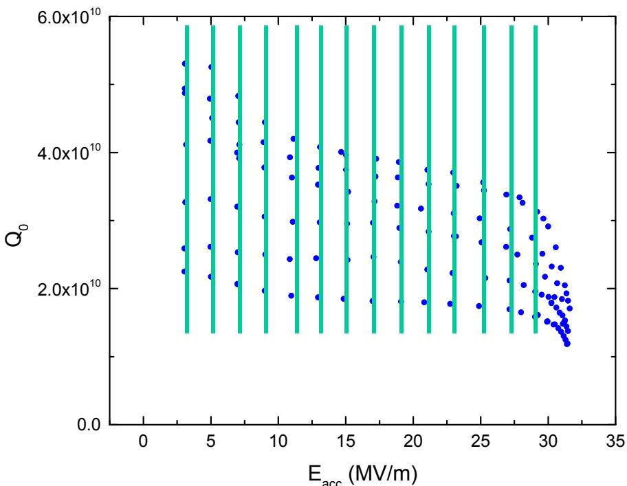
Measure  $Q(E_{acc}, T)$  at many different  $T < 2.17\text{K}$  and  $E_{acc}$
