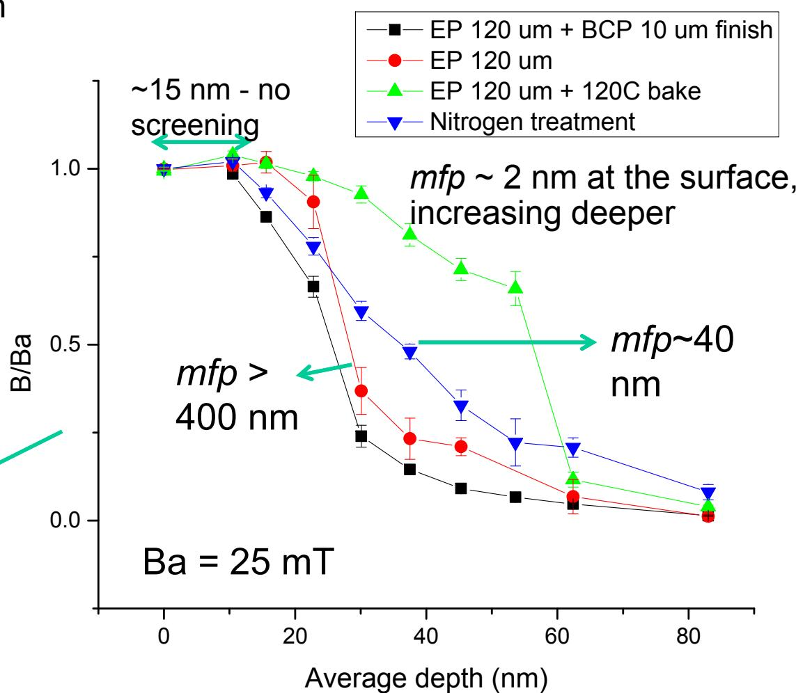
Fit by Gaussian model for the field at the muon site – approximate, qualitative comparison
