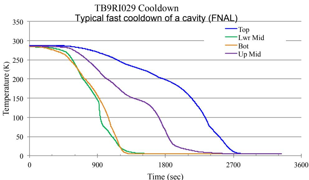
Integrate the H diffusion over the time spent in the precipitation temperature range  $T < 160\text{K} \Rightarrow L > 1\text{ um}$
