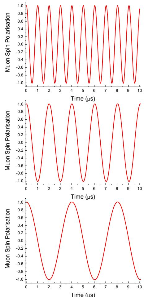
$$\omega_\mu(z) = \gamma_\mu B_{\text{loc}}(z)$$
