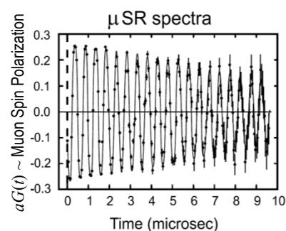
$$\omega_\mu(z) = \gamma_\mu B_{\text{loc}}(z)$$
