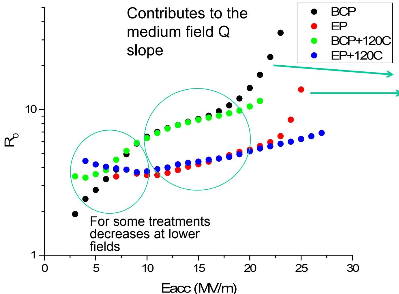
High field Q slope is clearly a residual resistance effect
