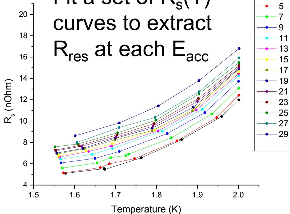
Can be fitted using both approximate formula  $R_{BCS}(T)=A/T \exp(-\otimes/kT)$ , and by more precise BCS calculation based on Halbritter's program – virtually no difference in the results
