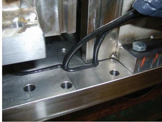
O-ring Inserted into Hood and Vacuum Vessel
