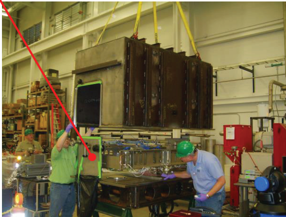
Vacuum Vessel Is Lowered on Baseplate
