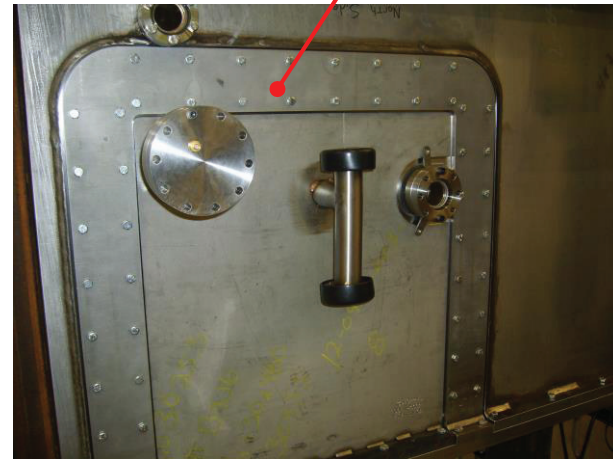
Seal Plate Presses O-ring to Vessel Assembly and Hood
