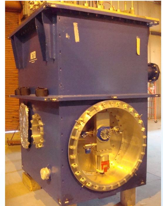
Assembled SRF gun cryomodule
