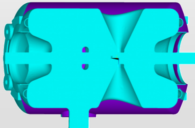
RF-Mechanical model: cavity with its helium vessel
