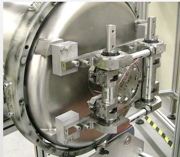
Prototype mounted on the triple Spoke cavity (Eucard) at IPNO
