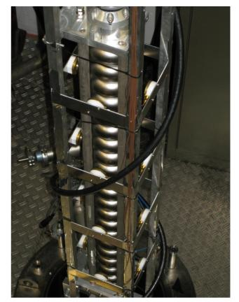
Figure 4: Darmstadt Quench Localization Set-Up. The OSTs are arranged around the cavity in four rings in order to cover the cavity completely giving the possibility of detecting quenches in every cell.
