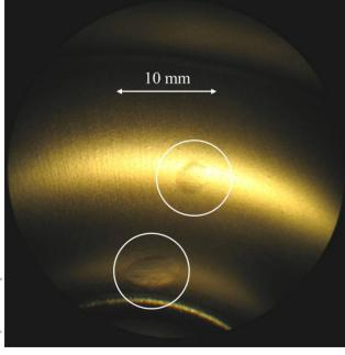
Figure 6: Defects close to the iris of cell #12, which has been identified to be the quenching cell using OST measurements.
