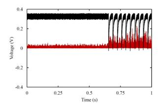
Figure 5: Typical graph of a series of quench events. The upper curve (black) shows the rf power coupled out of the cavity the lower curve (red) the detected OST signals.
