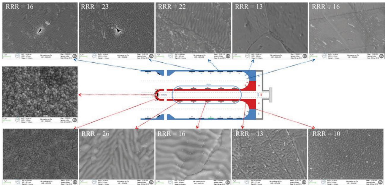
Figure 3: SEM pictures (magnification x10000) of niobium coated copper samples taken along the cavity outer conductor (in blue) and inner conductor (in red) and RRR measured at corresponding position, test #1, 52 mm top gap.
