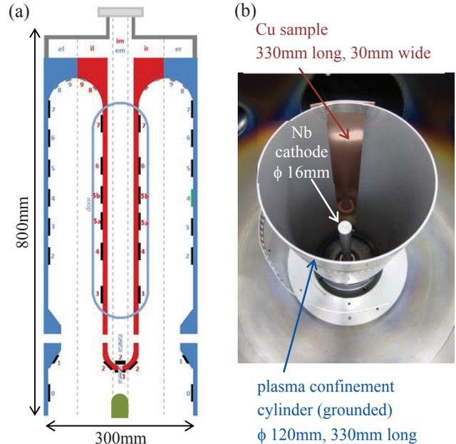
Figure 1: (a) cross section drawing of test cavity with position of samples, inner conductor in red, outer conductor in blue and centre electrode in green; (b) top view of the test bench setup with a copper band sample.
