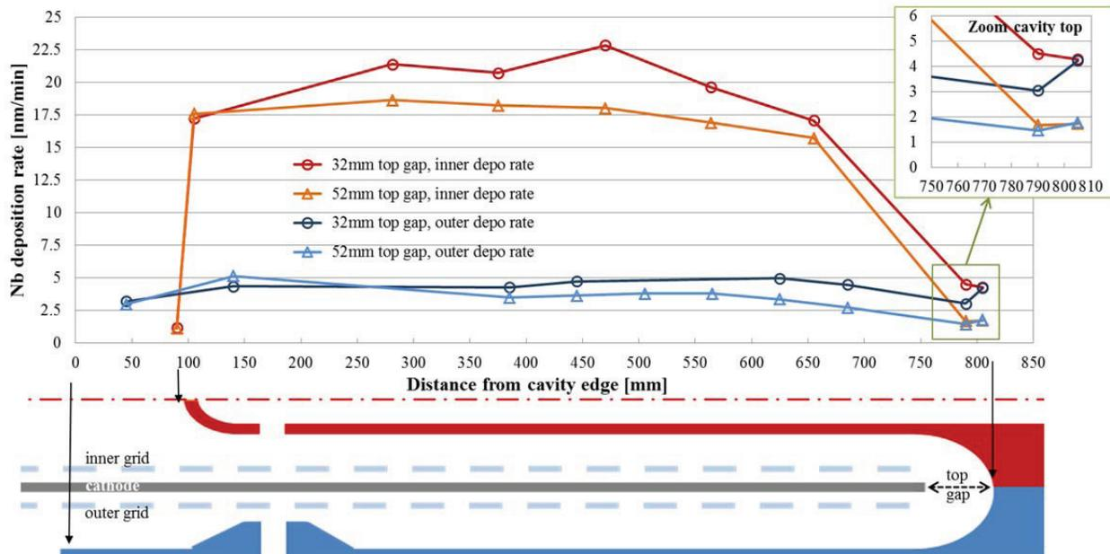
Figure 2: Niobium film deposition rates profiles along cavity outer conductor (in blue) and inner conductor (in red) for test #1 with top gap of 52 mm (Δ) and test #3 with top gap of 32 mm (O).
