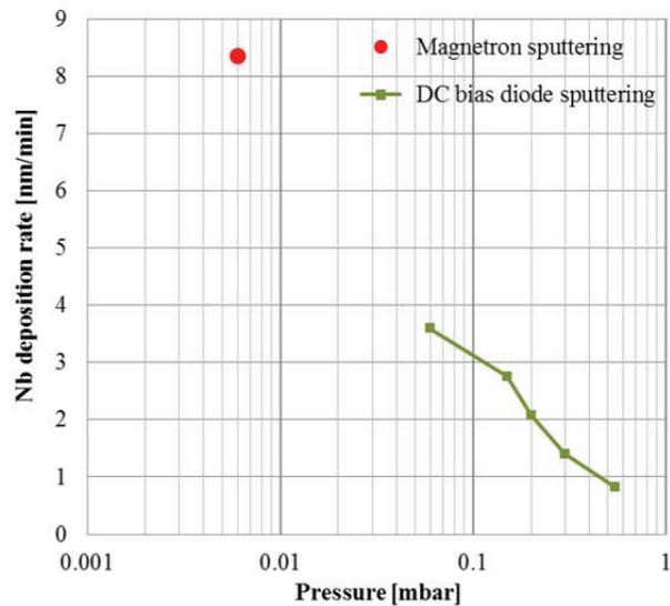
Figure 4: Average Nb film deposition rate from test bench study, as a function of pressure for the DC bias diode and magnetron sputtering, power = 155 W in both cases.
