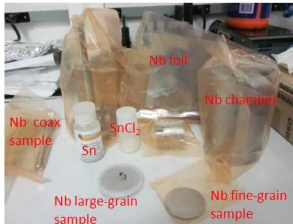
Figure 2: Components for Nb<sub>3</sub>Sn deposition on samples at Jefferson Lab.
