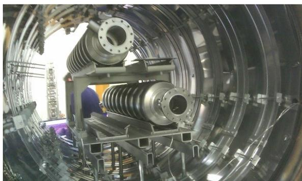
Figure 3: 800 C UHV oven loaded with two XFEL serial cavities.
