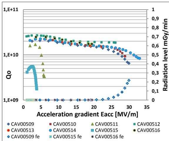
Figure 4: Test results of the eight pre series cavities made by Ettore Zanon.
