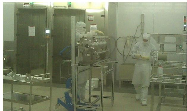
Figure 2: chemistry area inside ISO 7 cleanroom at EZ S.p.A. Left: closed loop BCP for BCP flash and outside etching.
