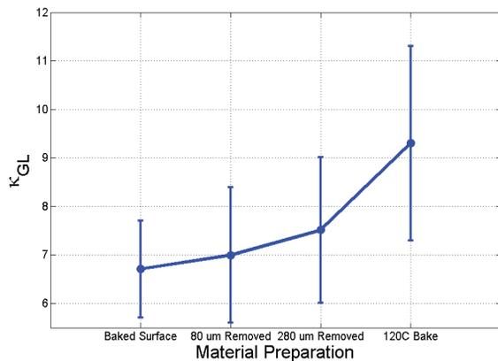
Figure 9:  $\kappa_{GL}$  as a function of material removal.
