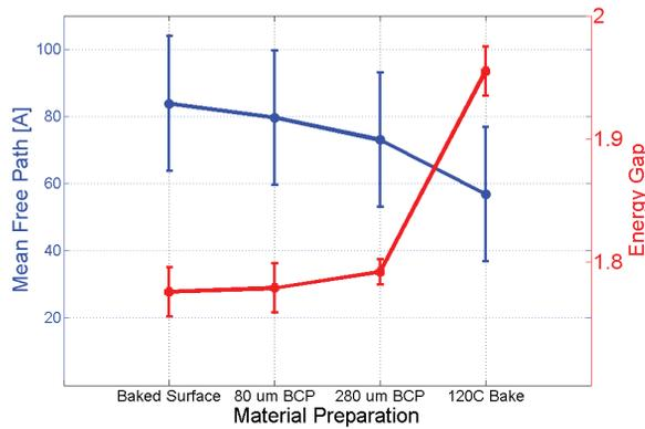
Figure 8: Mean free path and energy gap as a function of material removal.
