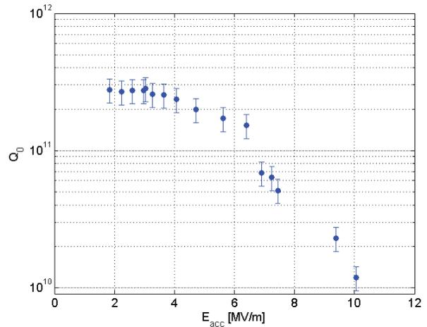
Figure 5:  $Q_0$  vs  $E_{acc}$  of the 1000°C heat treated surface at 1.42 K. The cavity obtained a record high  $Q_0$  of  $2.8 \times 10^{11}$  at 3 MV/m.
