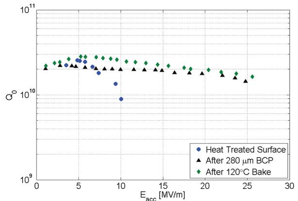
Figure 2:  $Q_0$  vs  $E_{acc}$  at 2.0 K for different amounts of material removal. Error bars on  $Q_0$  are 20% while error bars on  $E_{acc}$  are 10%.
