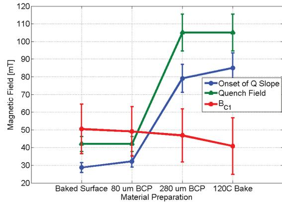
Figure 10:  $B_{c1}$ , onset of Q slope, and quench field (in units of maximum magnetic field) as a function of material removal.
