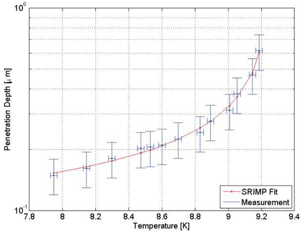
Figure 3: Fit of the penetration depth vs temperature using SRIMP to extract  $T_c$  and mean free path for the 1000°C heat treated surface.
