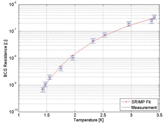
Figure 4: Fit of the BCS resistance vs temperature of the heat treated cavity using SRIMP to extract residual resistance and energy gap, using the values obtained from figure 3 for  $T_c$  and mean free path.
