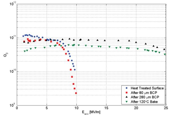
Figure 1:  $Q_0$  vs  $E_{acc}$  at 1.6 K for different amounts of material removal. Error bars on  $Q_0$  are 20% while error bars on  $E_{acc}$  are 10%.
