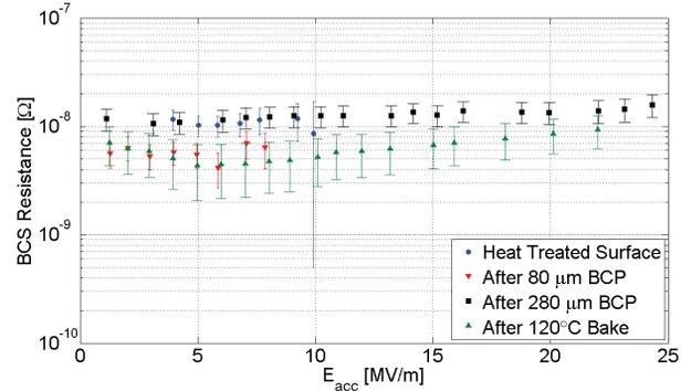
Figure 7: BCS Resistance as a function of accelerating field for different amounts of material removal. All tests were for 2.0 K except the 80  $\mu\text{m}$  removal which is at 1.8 K.
