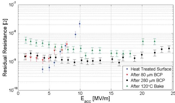
Figure 6: Residual resistance as a function of accelerating field for different amounts of material removal.
