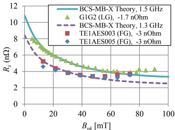
Figure 8: Field-dependent BCS surface resistance at 2.0 K, calculated by Xiao’s code and recent very low loss cavity test data from JLab at 1.5 GHz [8] and FNAL at 1.3 GHz [9] prepared by different methods.
