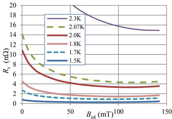
Figure 3: Effective 1.5 GHz surface resistance of standard Nb material parameters at various temperatures of interest.
