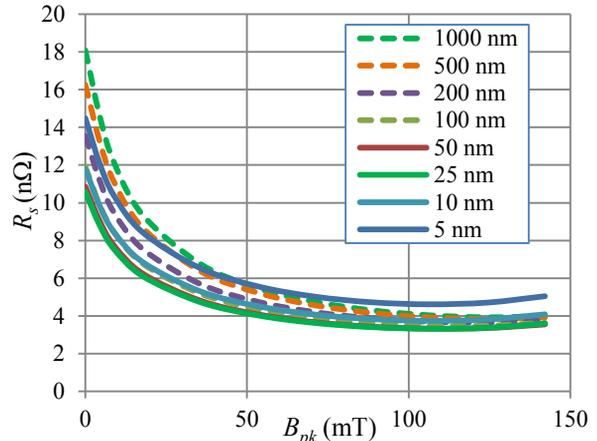
Figure 6: Effective 1.5 GHz surface resistance of Nb at 2.0 K with variations of electron mean free path.
