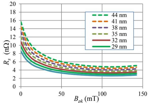
Figure 5: Effective 1.5 GHz surface resistance of Nb at 2.0 K with variations of London penetration depth  $\lambda_L$ .
