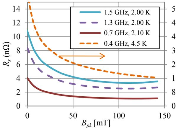
Figure 2: Calculated effective surface resistance under “standard conditions” for Nb versus peak RF magnetic field for 1.5 and 1.3 GHz at 2.0 K, 0.7 GHz at 2.1 K, and 0.4 GHz at 4.5 K.
