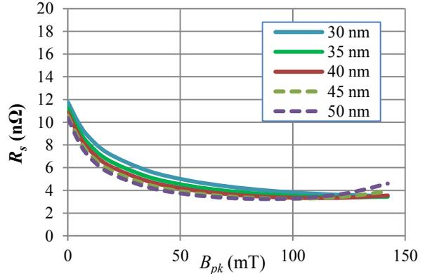
Figure 4: Effective 1.5 GHz surface resistance of Nb at 2.0 K with variations of coherence length  $\xi_0$ .
