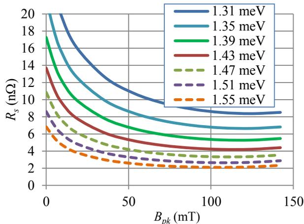
Figure 7: Effective 1.5 GHz surface resistance of Nb at 2.0 K with variations of the BCS energy gap,  $\Delta_0$ .
