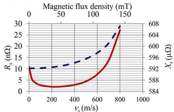
Figure 1: Surface resistance,  $R_s$ , (red line) and reactance,  $X_s$ , (blue dashed line) versus Cooper pair velocity for Nb at 2 K and 1.5 GHz.
