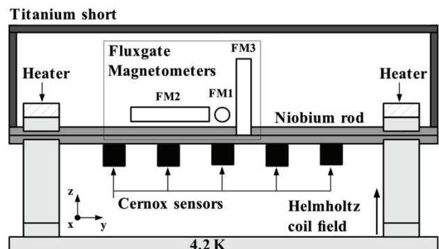
Figure 1: Experimental setup and positions of instruments.
