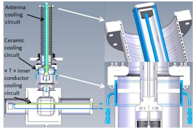
Figure 2: PC water cooling circuits
