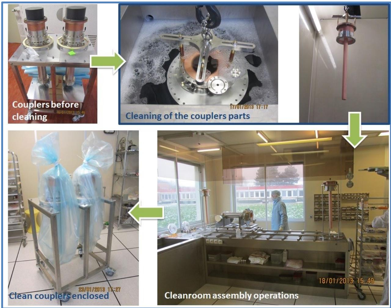
Figure 3: Cleaning and assembly of the PC prototypes.
