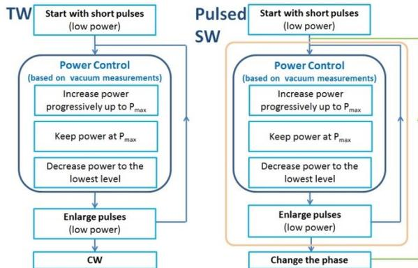
Figure 4: The RF conditioning sequence.  $P_{max}$  is the maximum RF power to reach.
