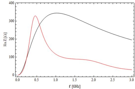
Figure 8: FB impedance at beam tube in red, ferrite alone in black.
