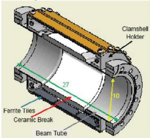
Figure 2: Ferrite plates over ceramic break (in cm)
