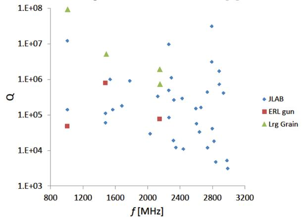
Figure 3: Cavity  $Q$ -values collected for the gun and the large-grain cavities at 2 K.
