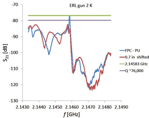
Figure 4:  $Q$ -measurement of the dipole 2.1458 GHz.
