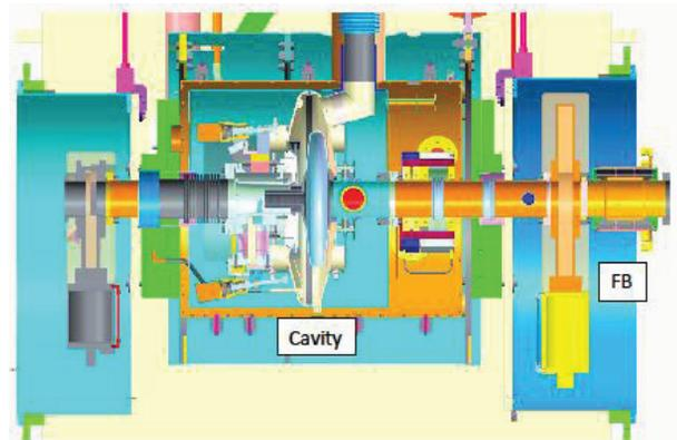
Figure 1: Ferrite break with gun cavity cryostat
