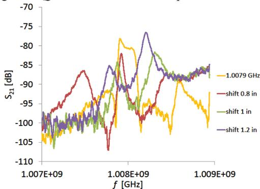
Figure 5: Shifting of the  $S_{21}$  curve by one FPC arm.
