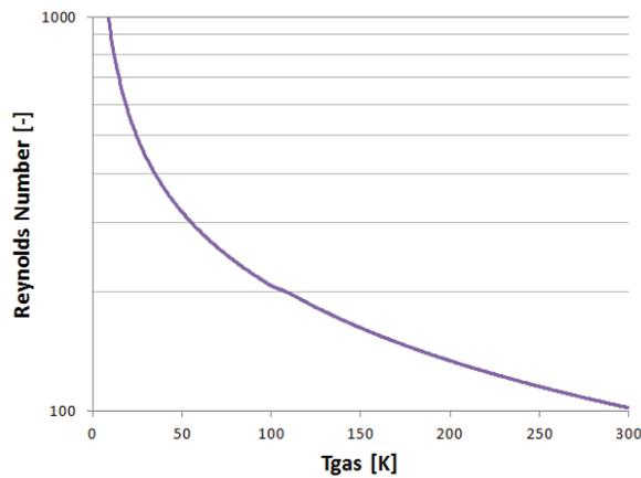
Figure 8: Reynolds Number versus gas temperature (for an equivalent channel hydraulic diameter of 2 mm; helium properties are calculated at 1.5 bar [7]).
