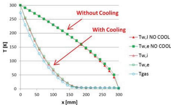
Figure 6: Static case, with and without cooling - Temperature profiles of internal (i) and external (e) walls, and helium gas along the DWT for non-cooled (filled markers) and cooled DWT (empty markers).
