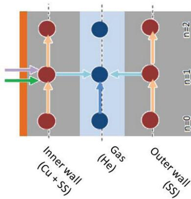
Figure 5: Heat exchange among elements of the mesh.
