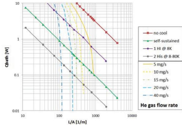
Figure 4: Heat transferred to a superfluid helium bath (300-2 K) as a function of geometry ratio  $L/A$ , and for different neck cooling techniques.
