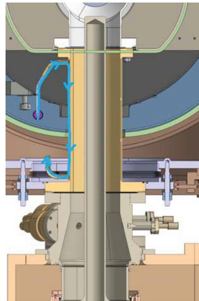
Figure 2: Cross section of the SPL power coupler with the helium channel for active gas cooling of the DWT.
