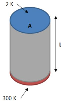
Figure 3: Simplified coupler geometry (neck):  $A$  is the cross section,  $L$  is the total length.
