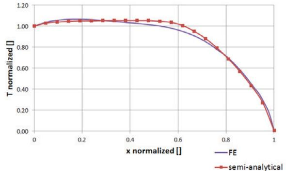
Figure 10: Dynamic case, without cooling - Normalised temperature profile comparison between finite elements and semi-analytical studies.
