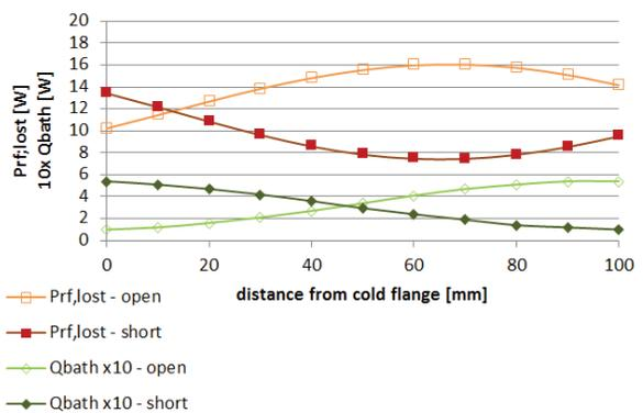
Figure 7: Dynamic case, with cooling - RF losses and thermal load to bath (x10, for better visualization) for different RF current configurations.
