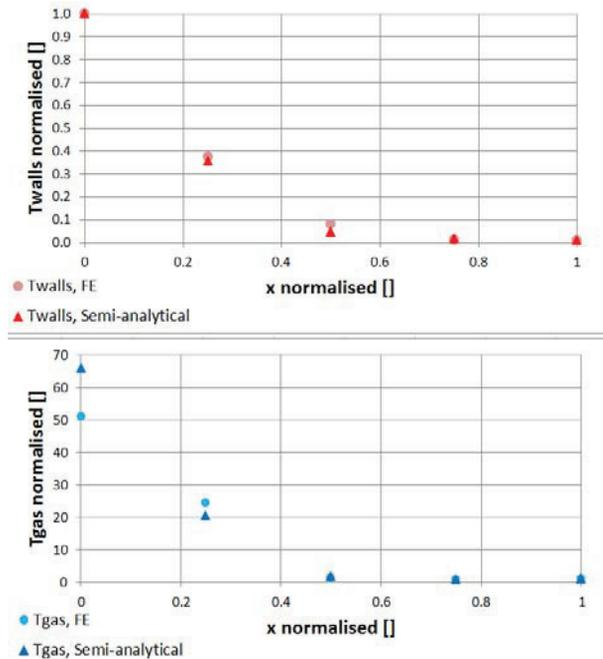
Figure 9: Static case, with cooling - Normalised temperature profiles comparison between finite elements and semi-analytical studies.
