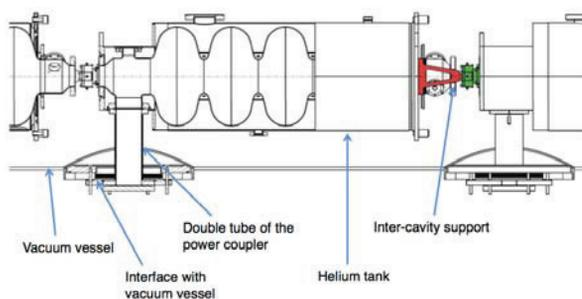
Figure 1: A sketch of the SPL cryomodule, with the RF power coupler and the intercavity support.
