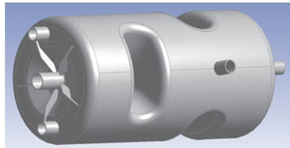
Figure 3: 3 mm cavity with 4 mm thick spokes and end cap stiffening ribs.
