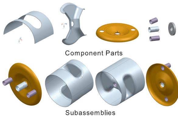
Figure 7: 500 MHz,  $\beta_0 = 1$  double spoke cavity fabrication planned parts.
