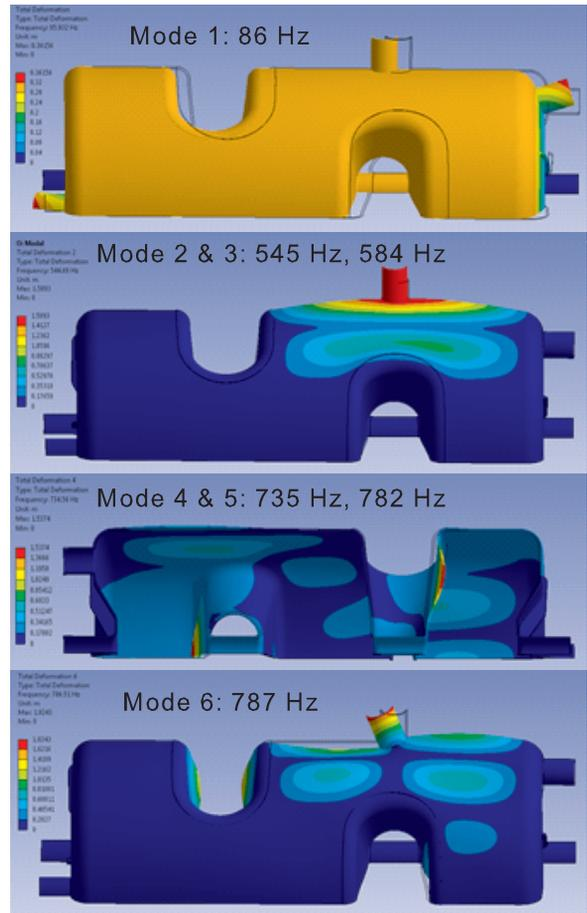
Figure 6: Cavity deformation due to the first six mechanical modes.
