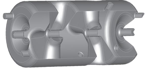
Figure 1: 500 MHz,  $\beta_0 = 1$  double-spoke cavity concept.
