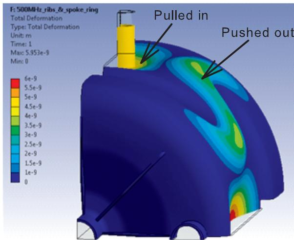
Figure 5: Cavity deformation due to LFD enhanced by a factor of  $4.1 \times 10^6$ .
