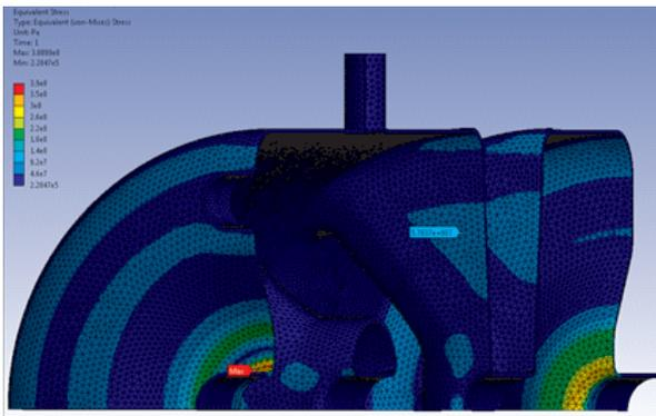
Figure 2: von-Mises stress under 2.2 atm, on the bare, 3 mm thick cavity, 4 mm spokes, with the beam pipes fixed.
