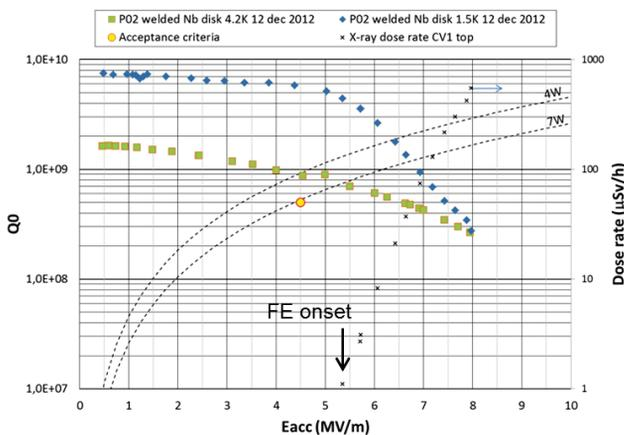
Figure 8: qualification test of the prototype 2:  $Q_0$  Vs  $E_{acc}$ .
