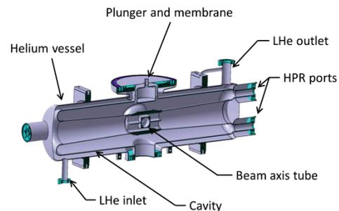
Figure 2: design of the HWR prototype
