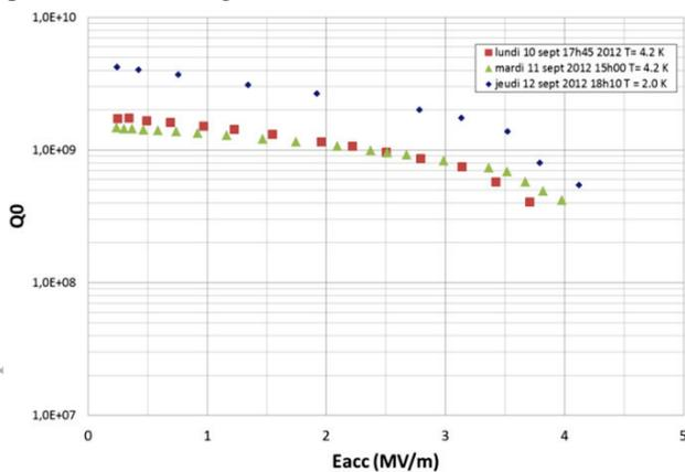
Figure 5: prototype 1 with inverted plunger:  $Q_0$  Vs  $E_{acc}$ .
