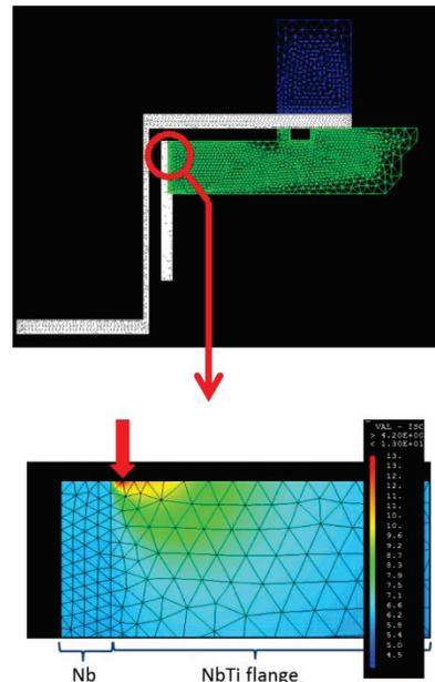
Figure 6: simulation on the NbTi flange with RF dissipation in the NbTi / Nb weld. Bottom: results for prototype 1. Top: the simulated geometry (white: the niobium plunger and part of the cavity body – green: the NbTi tuner flange).
