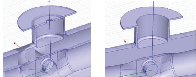
Figure 3: geometry of the proof-of-principle niobium plunger (right) compared to the original geometry (left).
