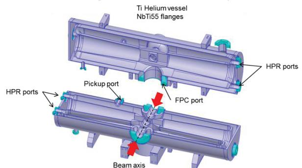
Figure 9: the new cavity design. The red arrow represents the force applied by the tuning system on the beam ports.
