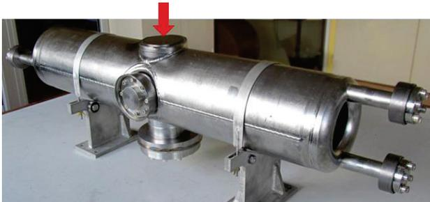
Figure 7: prototype 2 after the plunger port removal. The red arrow points on the welded niobium closing disc.
