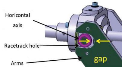
Figure 12: principle of the disengagement system.
