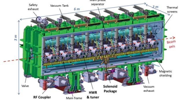
Figure 1: general layout of the LIPAc cryomodule
