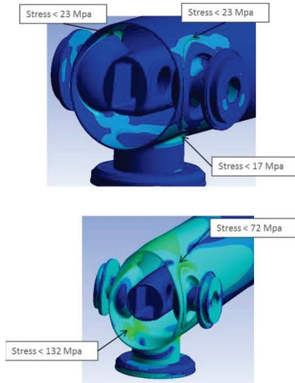
Figure 10: Von Mises stresses given by the finite element analysis. Top: ‘standard’ case – room temperature. Bottom: ‘operation’ case – liquid helium temperature.
