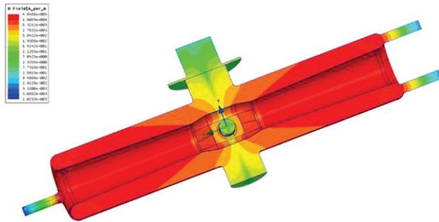
Figure 4: the inverted plunger setup: H-field is reduced by a factor of 25 on the NbTi tuner flange with respect to the original setup with the plunger.
