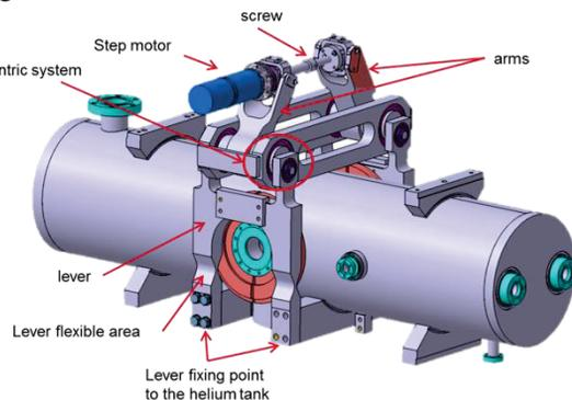
Figure 11: tuning system design.
