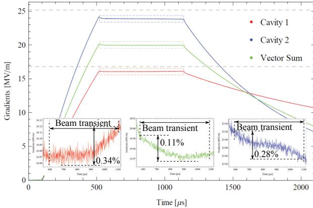
Figure 5: Cavity 1, cavity 2, and vector sum gradients [MV/m] versus time [s] during  $P_k Q_L$  operation. The dashed lines indicate virtual quench limits of 16.8 MV/m and 25.2 MV/m.
