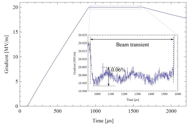
Figure 3: Vector sum gradient [MV/m] versus time [s] during high  $Q_L$  operation.
