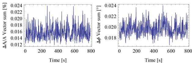
Figure 7: Vector sum gradient and phase stabilities during beam transient versus time [s].
