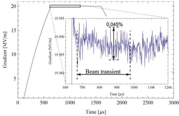
Figure 2: Vector sum gradient [MV/m] versus time [s] during nominal operation.
