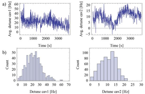
Figure 4: a) Detune [Hz] of both cavities versus time [s] and b) detune histogram for both cavities during high  $Q_L$  operation.
