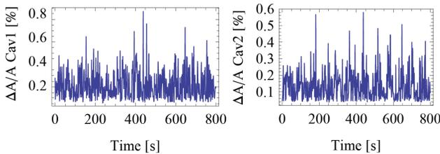
Figure 6: Cavity 1 (left) and cavity 2 (right) gradient stabilities during beam transient versus time [s] in  $P_k Q_L$  operation.
