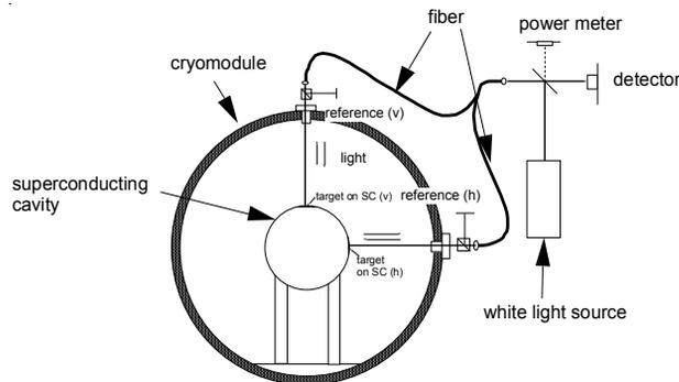
Figure 2: Schematic drawing of WLI monitor setting to cryomodule.
