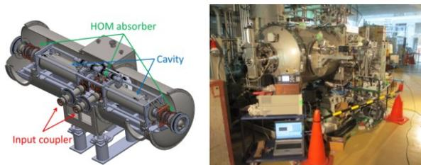
Figure 8: (Left) Schematic view of cERL main linac cryomodule (Right) Picture of cERL main linac cryomodule at cERL beam line.
