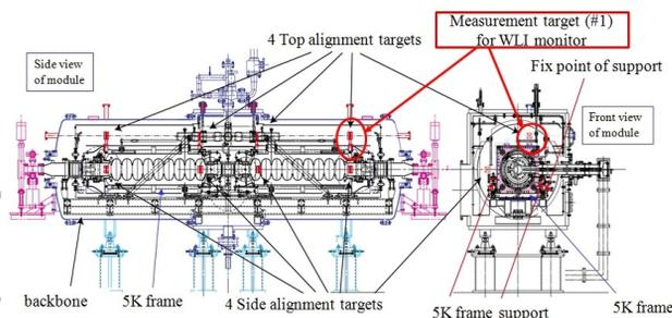
Figure 9: Detailed cross sections of the cERL main linac cryomodule with 8 alignment targets including the target (#1) for WLI monitor.
