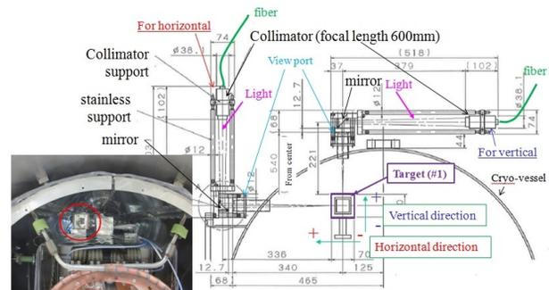
Figure 10: Setup of WLI monitor around cERL main-linac cryomodule. Red circle in the picture shows the optical target (#1) used for WLI monitor.
