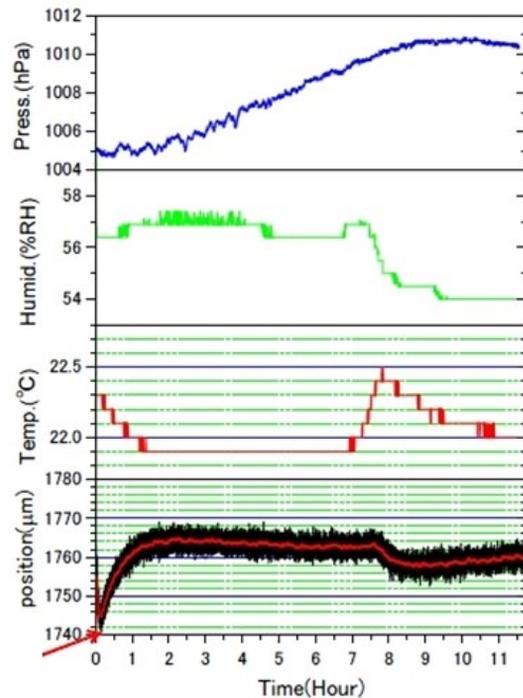
Figure 7: Long-term stability of the WLI monitor.
