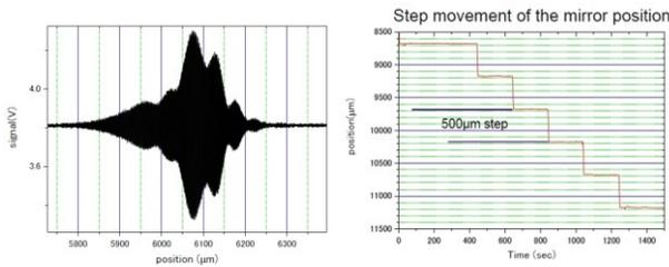
Figure 5: (Left) Measured interference pattern at a test stand. (Right) measured peak position of the interference pattern by changing the reference scanner.
