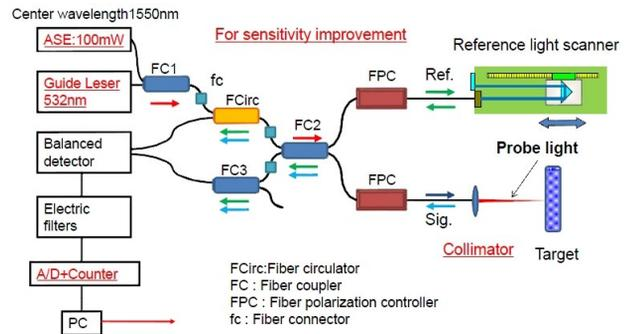
Figure 3: Setup of the WLI monitor at a test stand.
