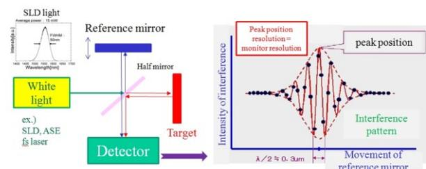
Figure 1: Principle of the WLI position monitor.
