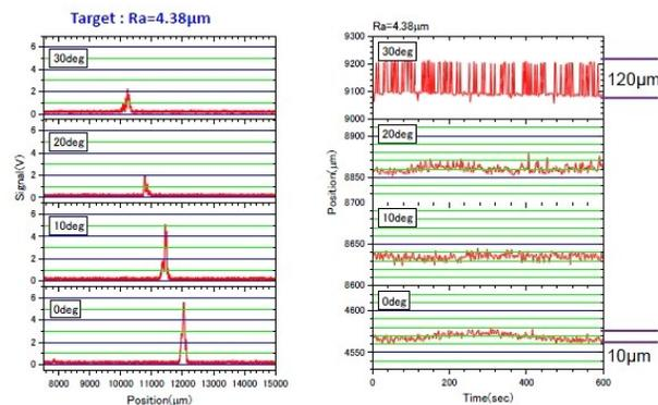
Figure 6: (Left) Measured interference pattern with the different incident angle. (Right) measured stability of the peak position of the different incident angle for 10 min.
