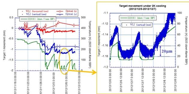
Figure 11: (Left) Measurement results of the movements of target #1 together with the 5K frame temperature (Right) Expanded view of the measurement results of left figure in orange circle. The left and right vertical axes of both figures show the measured target movements and the measured temperature of 5K frame, respectively.
