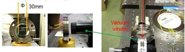
Figure 4: Picture of the setup from the collimator to the target of WLI monitor at the test stand.
