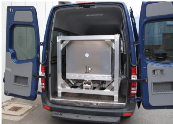
Figure: 4 View to the Transport Frame for the Transport of BQU's.
