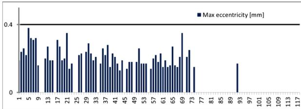
Figure 4: Maximal value of cavity eccentricity before welding in helium tank.
