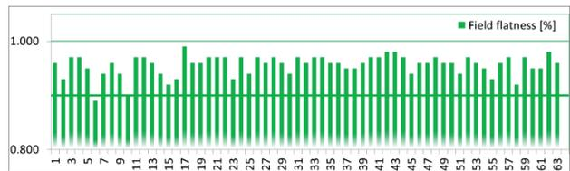
Figure 6: Cavity field flatness at TM010 pi-mode before BCP.
