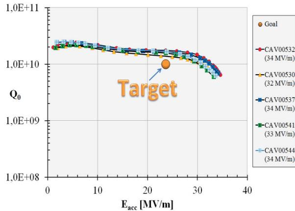
Figure 8: Vertical test result of some cavities.
