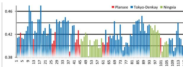
Figure 2: Shrinkage of equator welding for different materials.
