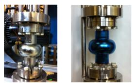
Figure 10: A 6 GHz cavity with a standard external surface (left). The same cavity after the RF test has been anodized only externally (right) and then re-measured. What is important to consider is that such operation is done when keeping the cavity on the stand always under U.H.V.
