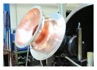
Figure 12: Layout of the pieces for electron beam weld of the iris.
