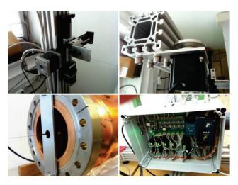
Figure 27: Automated bead-pull test stand for SPL cavities.
