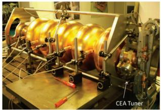
Figure 31: Tests of cavity deformation during tuning with CEA Saclay cold tuner.
