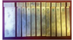
Figure 25: Nb - SS brazed samples for chemical testing.
