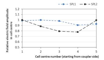
Figure 28: Bead-pull results of the SPL copper mock-ups.
