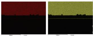
Figure 23: EDS qualitative analyses showing higher concentration of Cr an Fe in the Nb – Cu interface.
