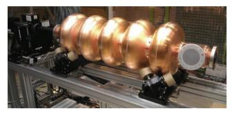
Figure 37: Optical inspection bench.
