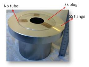
Figure 20: Layout of the pieces before the brazing operation.
