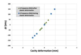
Figure 30: Measured Pi-mode frequency change vs. mechanical deformation of cell no 4.
