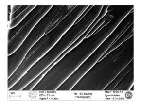
Figure 24: Fractography of the Nb - Cu interface observed in the Nb side.
