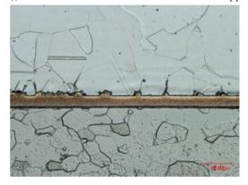
Figure 21: Metallographic observation of the brazed joint with Stainless steel on top, copper in the middle and niobium in the bottom.
