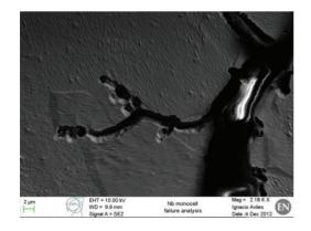
Figure 18: SEM image of one of the branches of the cross section of the defect.
