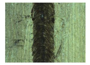
Figure 38: Equator welding inspection of copper cavity.
