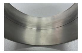
Figure 16: Material defect observed after machining of the surface.
