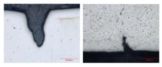
Figure 15: Metallographic observation of a defect found in the inner surface, submitted to electropolishing (left), and in the outer surface, not submitted to electropolishing (right).
