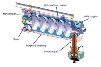
Figure 5: SPL  $\beta$ =1 cavity with helium tank, tuner, main coupler, HOM coupler to be tested at CERN in cryo-module.
