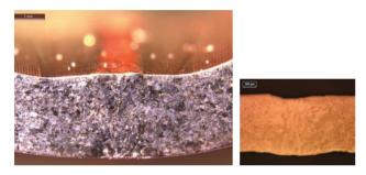
Figure 13: Metallography of a weld cross section of the iris (left) and equator (right).
