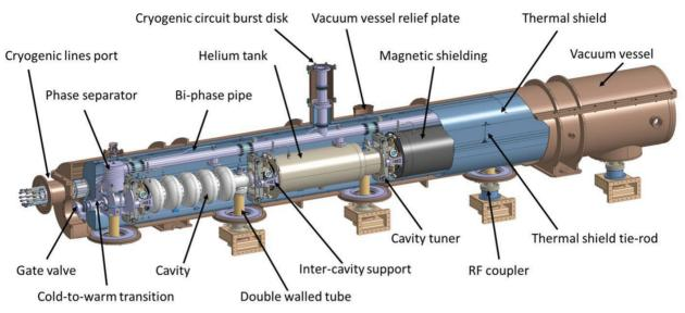
Figure 3: General Assembly View of the SPL Short Cryo-module (courtesy of IPN Orsay).
