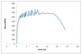
Figure 6: Tensile test on niobium sample from Supplier A plate 2 at 4.2 K.
