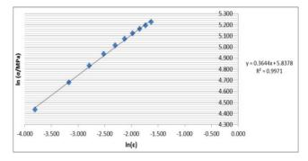
Figure 8: True stress vs. true strain curve in a logarithmic scale used for the determination of *n*.
