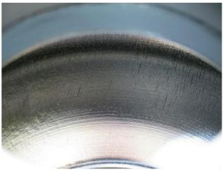
Figure 36: Niobium surface after 220 microns removal by electropolishing.
