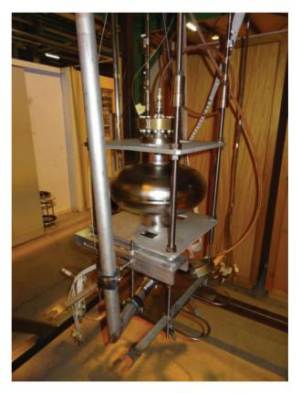
Figure 40: Vertical cryostat for cavity cold test.
