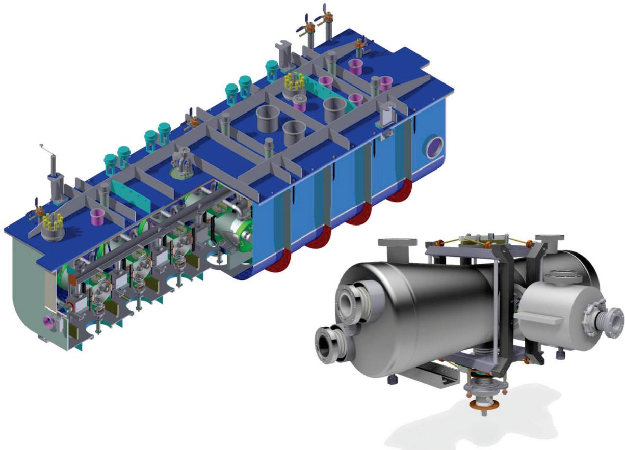
Figure 3: Project-X half-wave resonator cryomodule model. The cryomodule contains 8 superconducting 162.5 MHz,  $\beta = 0.112$ , half-wave resonators and 8 superconducting solenoids with beam position monitors rigidly attached to each solenoid. (Top) The cryomodule with a section cut out to show the inside. (Bottom) A single focusing period containing a solenoid, beam position monitor and half-wave resonator.
