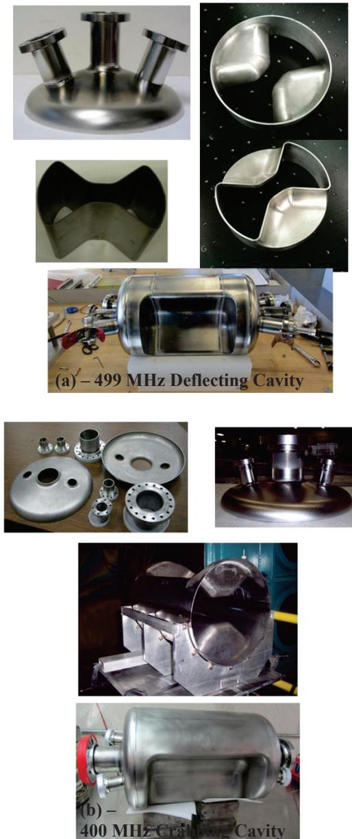
Figure 3: Fabrication of (a) 499 MHz and (b) 400 MHz rf-dipole cavities.
