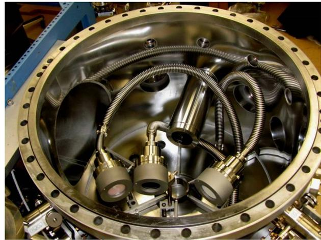
Figure 2: Setup in the UHV multi-technique deposition system main chamber.
