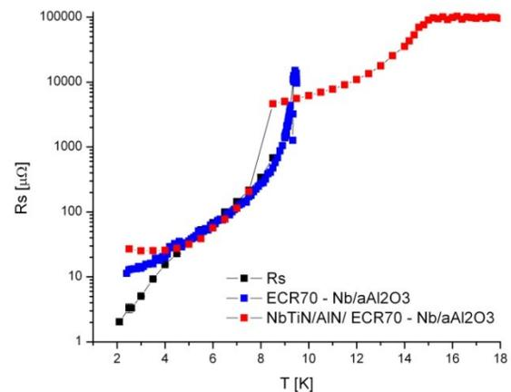
Figure 4: Surface resistance as a function of temperature for NbTiN/AlN structure coated on ECR Nb film measured in the SIC setup.
