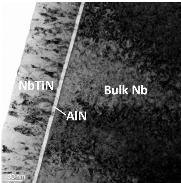
Figure 5: TEM image of a FIB cut NbTiN/AlN/Nb structure.
