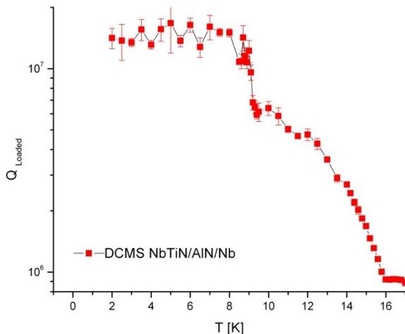
Figure 6: Quality factor as a function of temperature for NbTiN/AlN/Nb (bulk) measured in the SIC setup.
