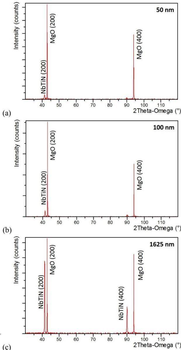
Figure 3: XRD Bragg-Brentano ( $\theta$ - $2\theta$ ) spectra for NbTiN coated on MgO (100) with a thickness of (a) 50 nm, (b) 100 nm and (c) 1.6  $\mu\text{m}$ .
