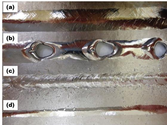
Figure 6: Examples of underbeads. (a) Full penetration weld without spatters. (b) Weld bead with holes. (c) Underbead with spatters. (d) Narrow underbead.
