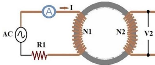
Figure 2: B-H curve measurement method by ASTM.
