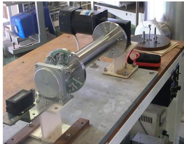
Figure 10: Completed bobbin for 8 T 25 cm main solenoid.
