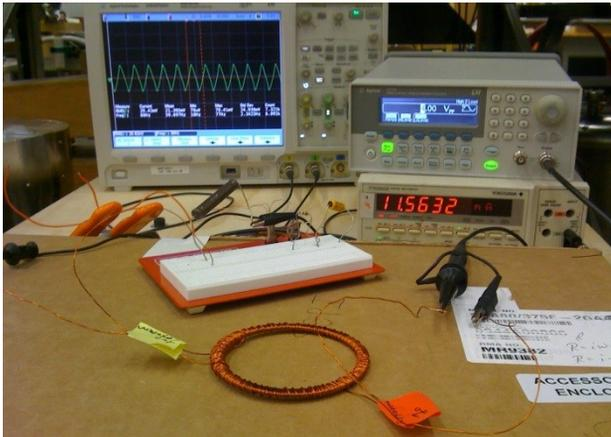
Figure 1: B-H curve measurement system at room temperature.
