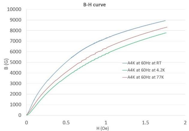
Figure 3: B-H curve at RT, 77 K, and 4.2 K for A4K material.
