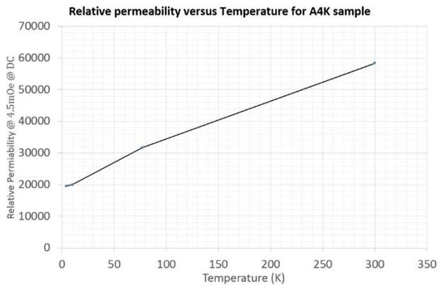
Figure 5: Temperature dependence of  $\mu$  at 4.5 mOe with A4K material.
