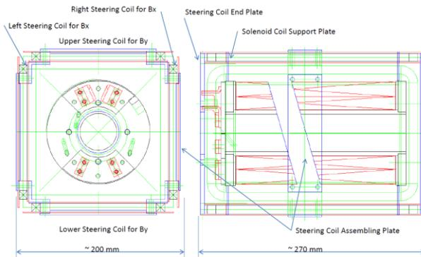
Figure 9: 8 T 25 cm solenoid cold mass with steering dipole coils.
