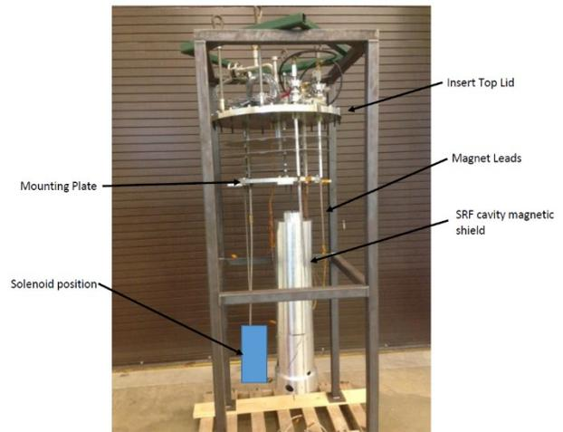
Figure 7: A magnetic shielding insert for magnetic attenuation measurement at cryo-temperatures.
