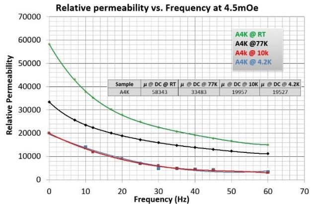
Figure 4: Frequency dependence of relative permeability ( $\mu$ ) at 4.5mOe for A4K material at RT, 77K, 10K, and 4.2K.
