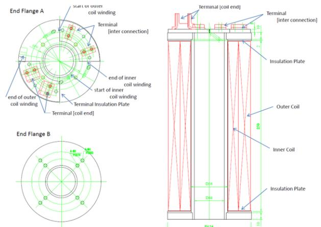
Figure 8: 8 T SC 25 cm main solenoid design.
